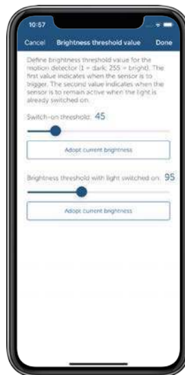
Figure 45: Screenshot Configuration group with motion detector / presence sensor
