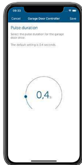
Figure 59: Screenshot garage door controller pulse duration
