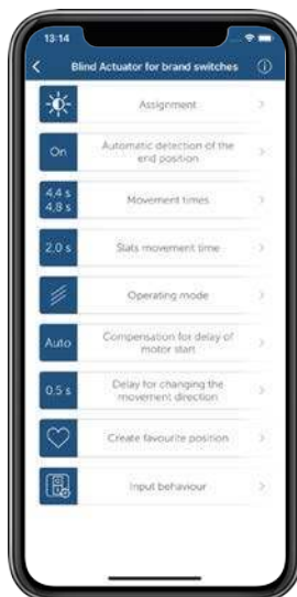
Figure 30: Screenshot Device settings shutter and blind actuators
