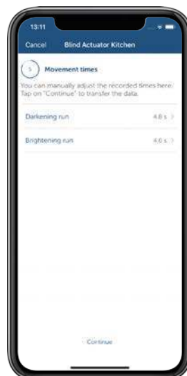
Figure 29: Screenshot Adjusting movement times manually
