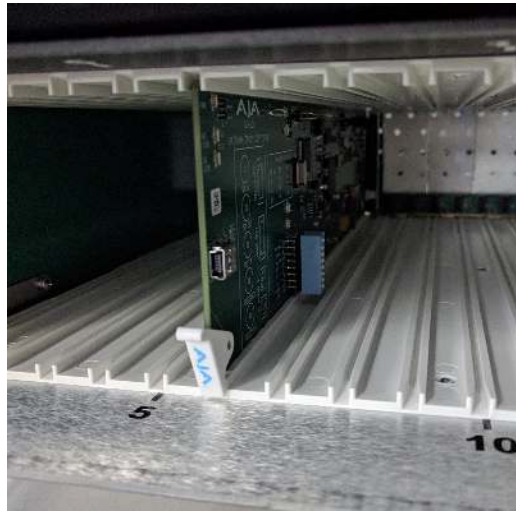
Figure 8. OG-4K2HD card inserted Into Right Slot
