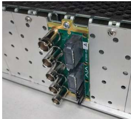
Figure 7. Rear Card Inserted Into Frame Seating Slot
