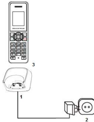
Figure 6: Setting up the charger station
