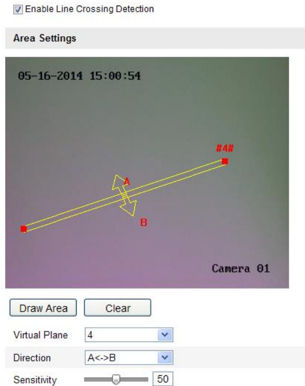
Figure 6-60 Draw Crossing Line
