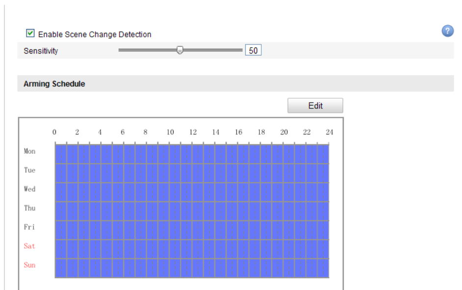
Figure 6-58 Configuring Scene Change Detection
