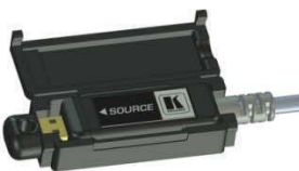
I: Place the micro HDMI connector inside the Pulling Tool.
