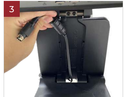
3 Pull the cable through the cable tray.
