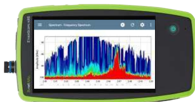
Frequency Spectrum App on the EtherScope nXG
