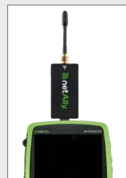
Optional NXT-1000 Portable Spectrum Analyzer for 2.4/5GHz.
