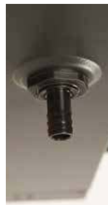
Condensation-water discharge fittings
