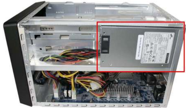
Use of the power supply FSP300 in the Shuttle XPC cube SH610R4
