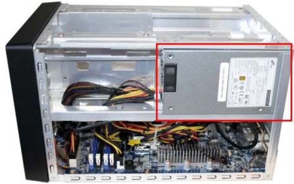
Use of the power supply FSP500 in the Shuttle XPC cube SH570R8
