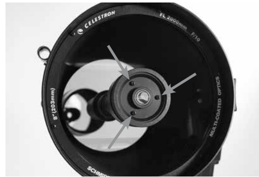
Secondary Mirror Collimation Adjustment Screws
