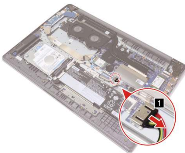
Figure 25. Disconnect the battery pack cable
