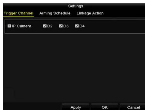
Figure 5. 18 Set Trigger Camera of VCA Alarm
