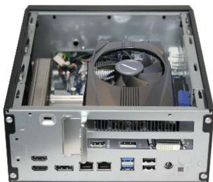
Shuttle XPC slim Barebone XH610G2 with powerful graphics card installed
