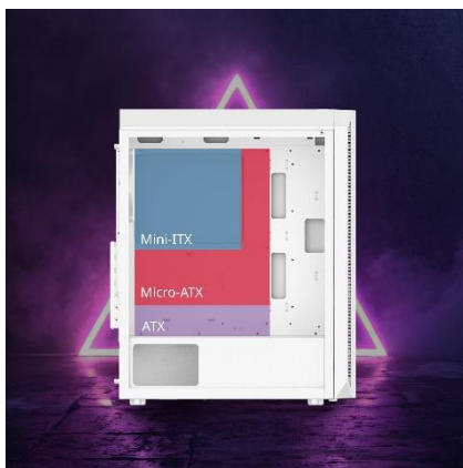
Supports Mini-ITX, Micro-ATX, and ATX Motherboards
