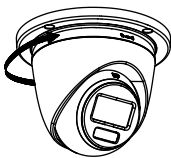
Figure 2-25 Snap Camera into Installation Plate
