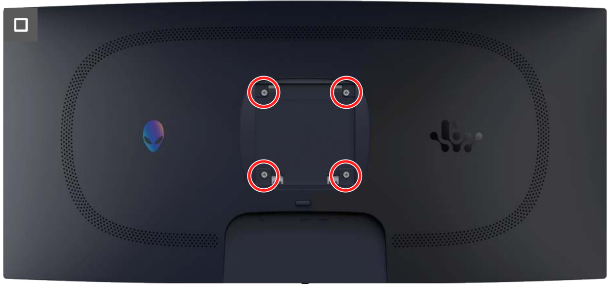
Figure 19. Installing the back cover
