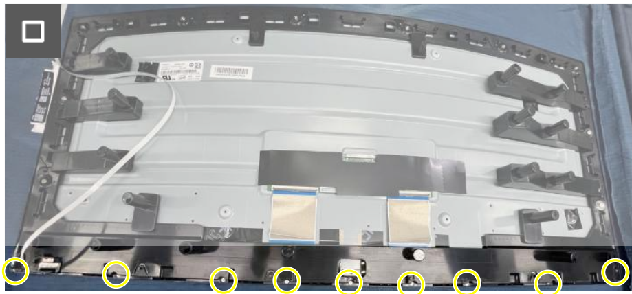
Figure 36. Removing the middle frame
