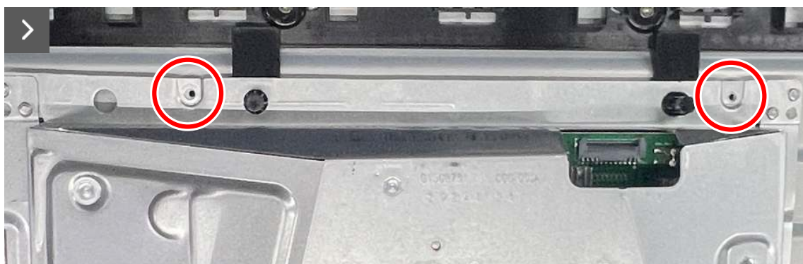
Figure 22. Removing the metal shield
