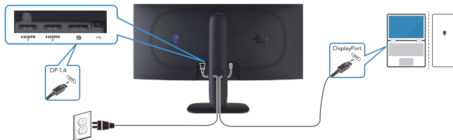
Figure 8. Connecting the DisplayPort (DP to DP) cable
