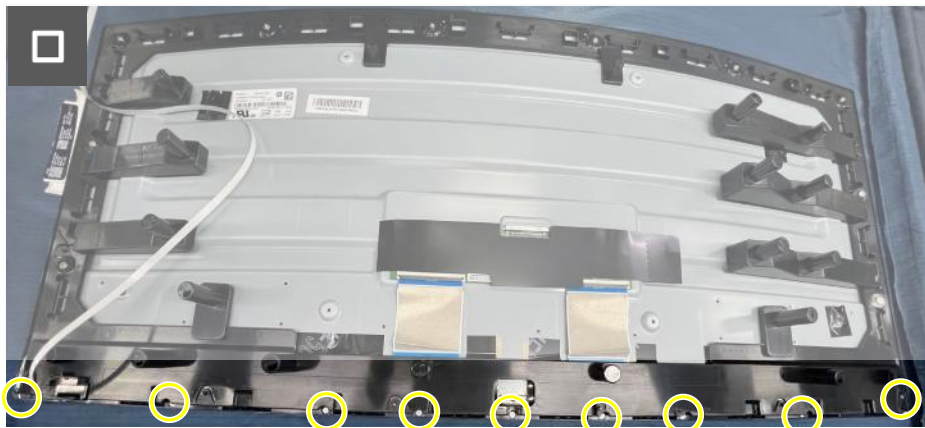
Figure 37. Installing the middle frame
