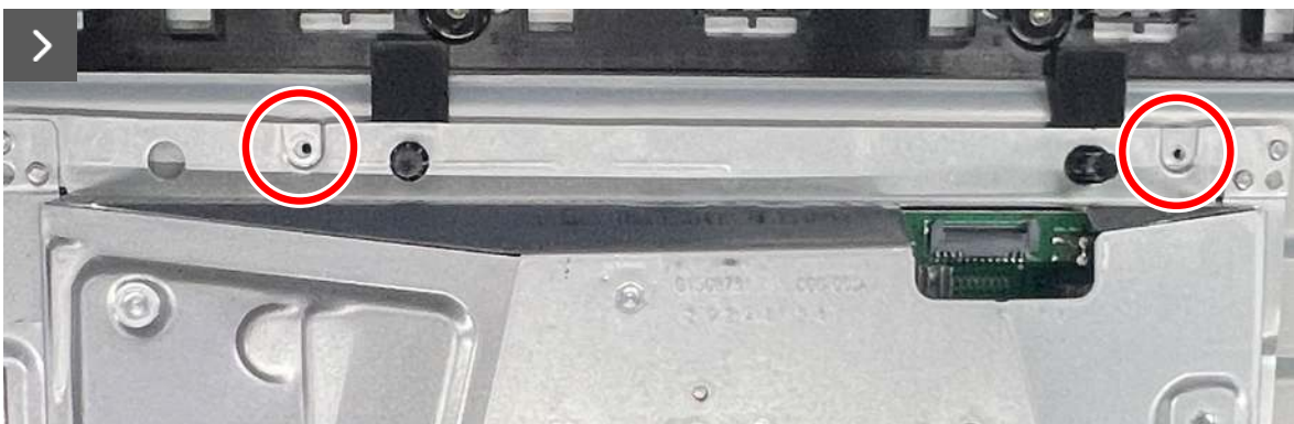
Figure 26. Installing the metal shield
