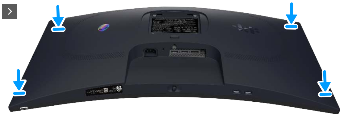
Figure 18. Installing the back cover
