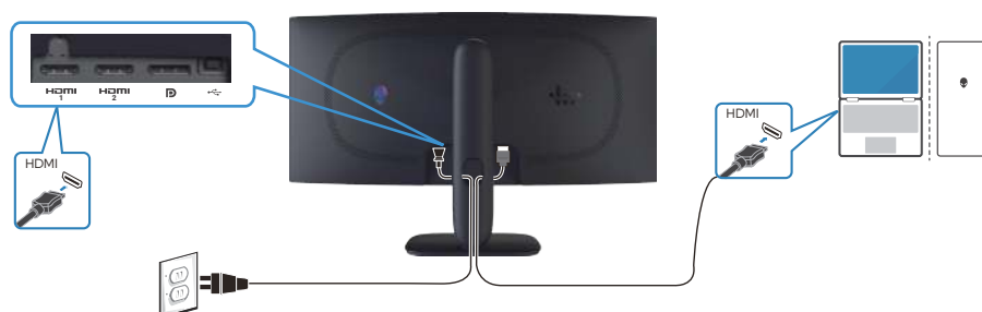
Figure 9. Connecting the HDMI cable
