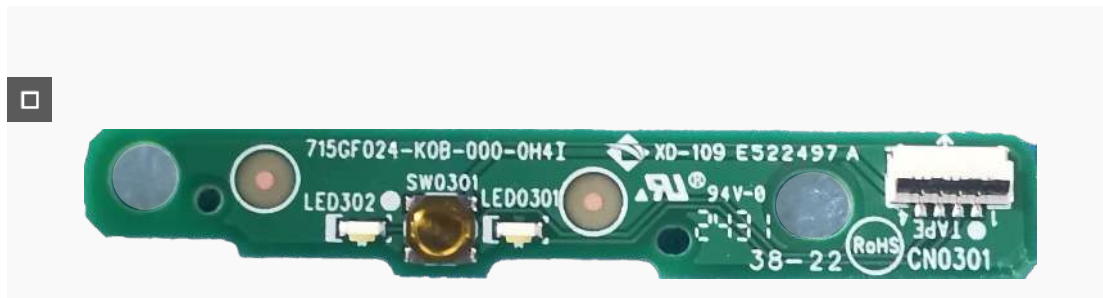
Figure 39. Removing the power-button board
