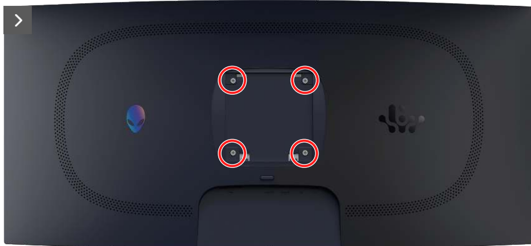
Figure 13. Removing the back cover
