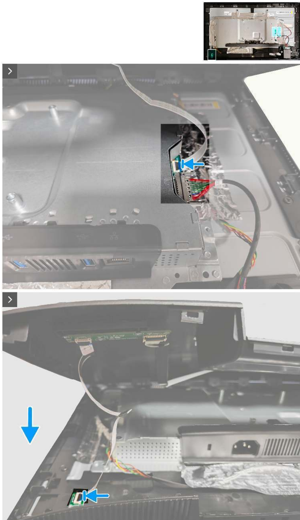
Figure 13. Installing the back cover
