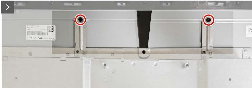
Figure 23. Installing the metal frame
