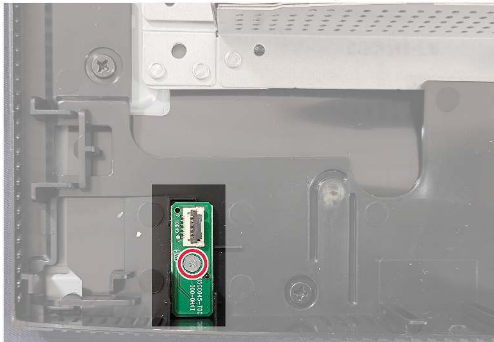
Figure 18. Installing the LENS board
