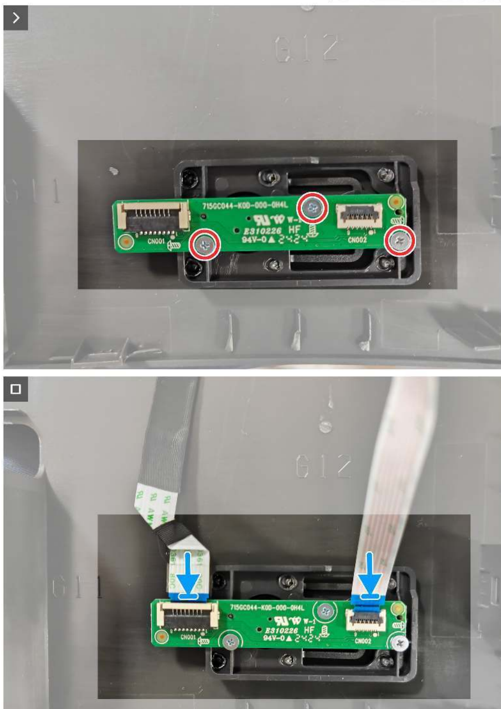
Figure 16. Installing the keypad board
