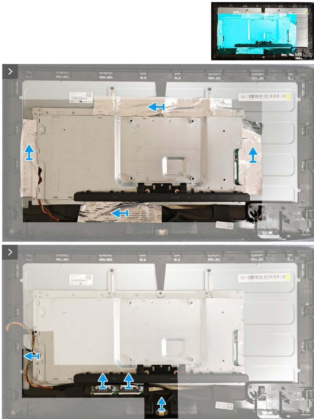
Figure 21. Removing the metal frame
