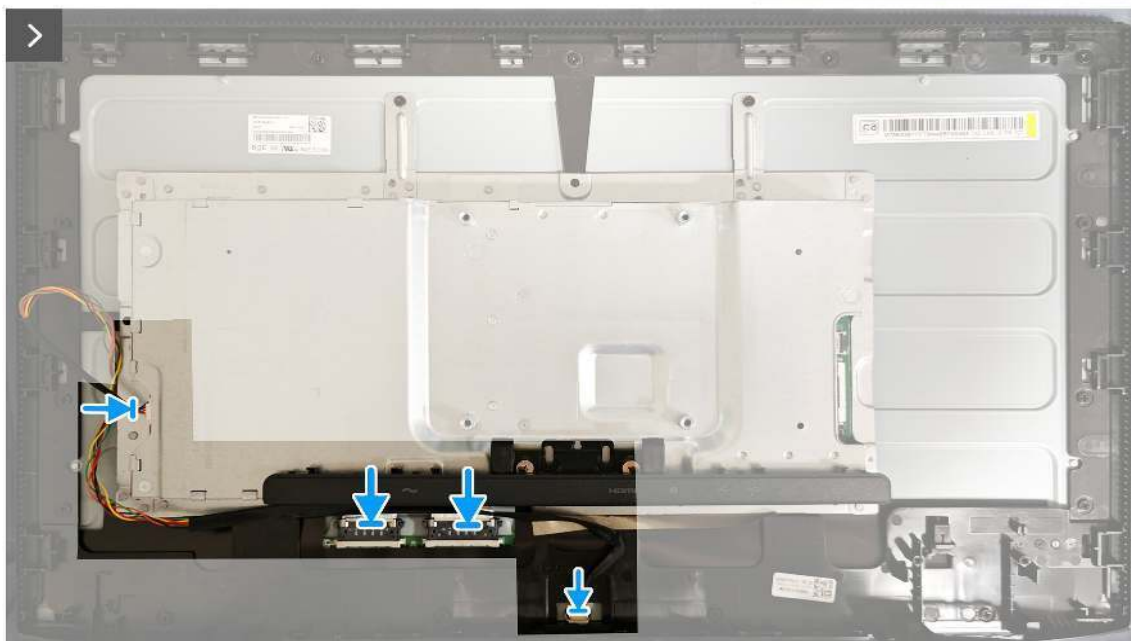
Figure 24. Installing the metal frame
