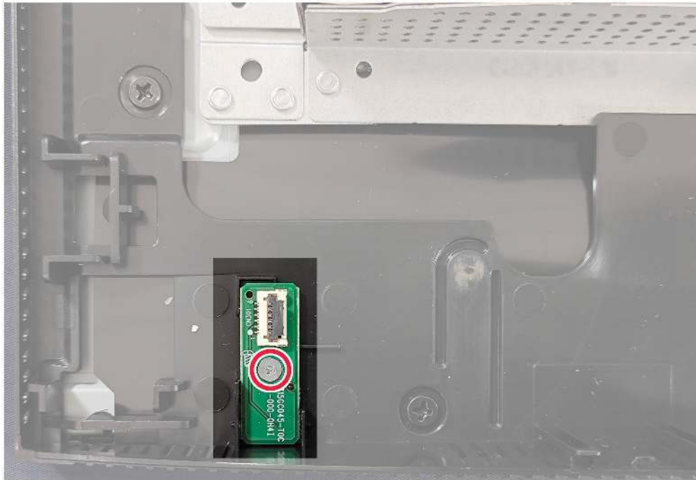
Figure 17. Removing the LENS board
