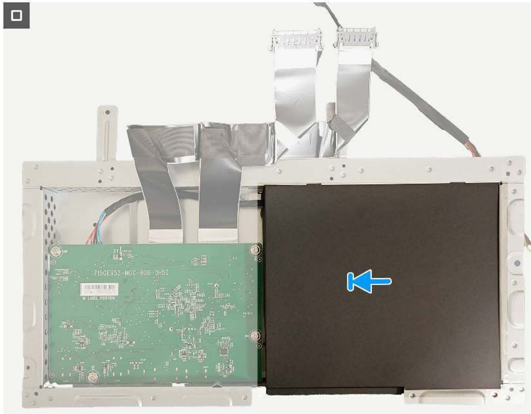
Figure 30. Installing the system board and power board
