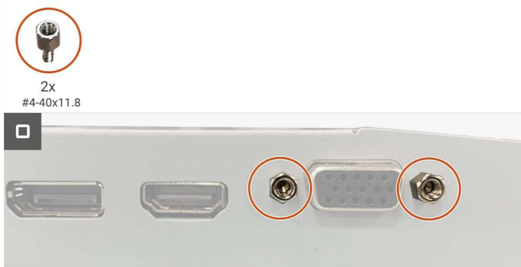
Figure 27. Installing the interface board
