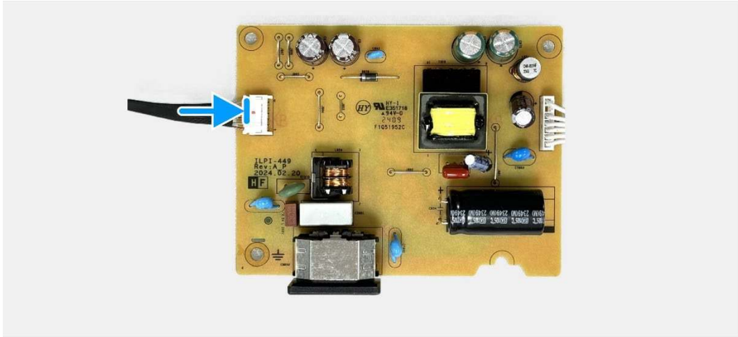
Figure 31. Installing the power board
