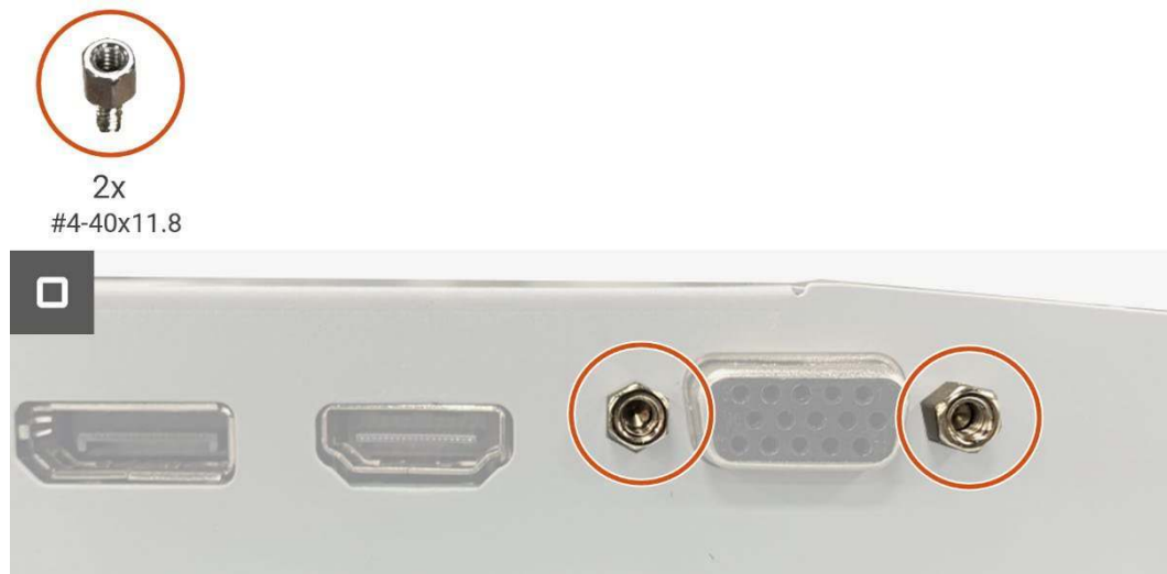
Figure 51. Installing the interface board
