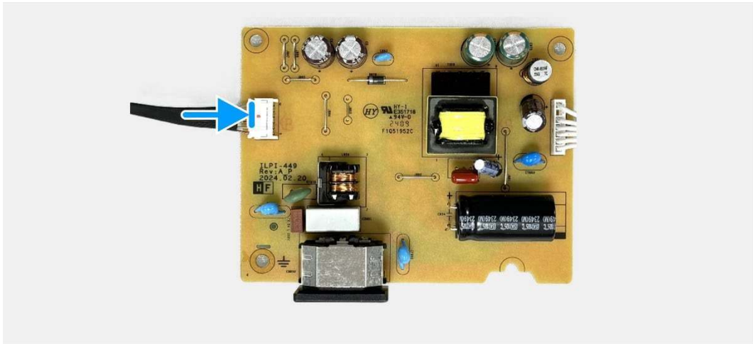
Figure 53. Installing the power board
