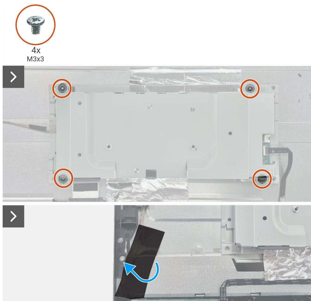
Figure 40. Removing the chassis assembly
