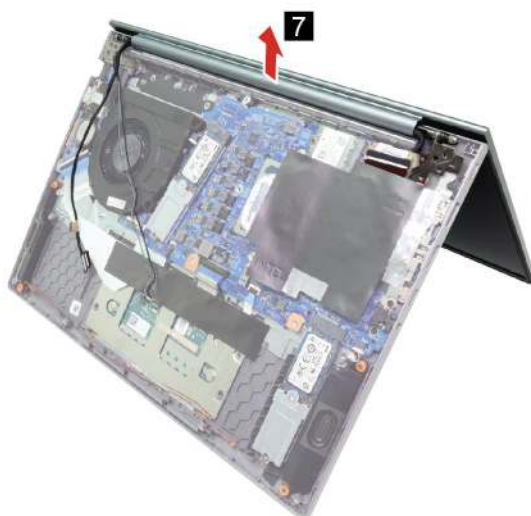
Figure 37. Rotate and remove LCD module
