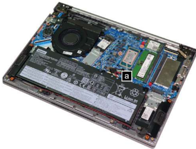
Figure 5. Areas on the system board where thermal interface materials are applied
