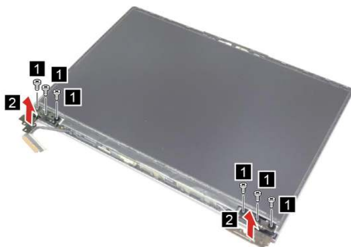
Figure 40. Remove six screws and remove the hinges
