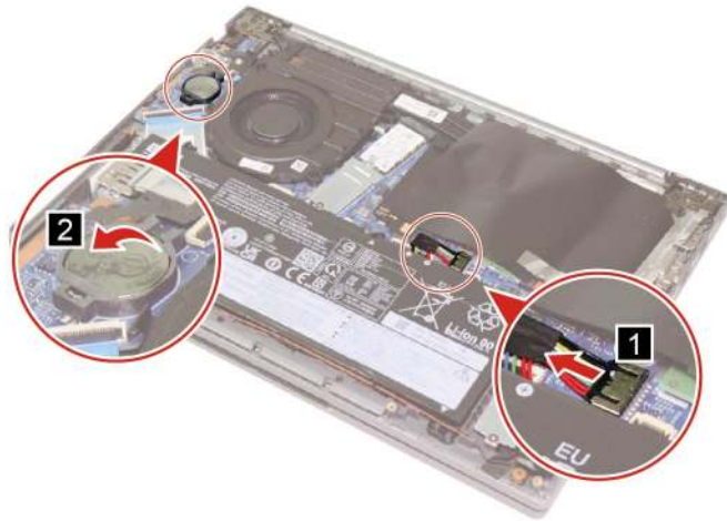
Figure 19. Remove the coin-cell battery
