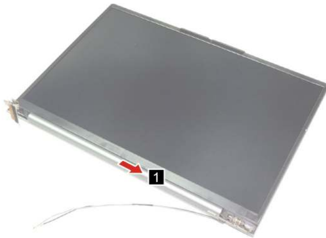
Figure 38. Remove the hinge cover
