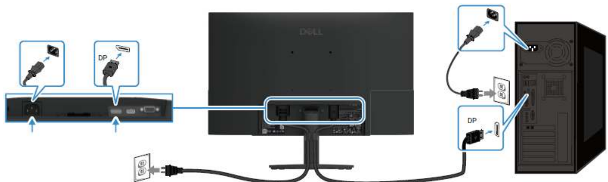
Figure 9. Connecting DP cable
