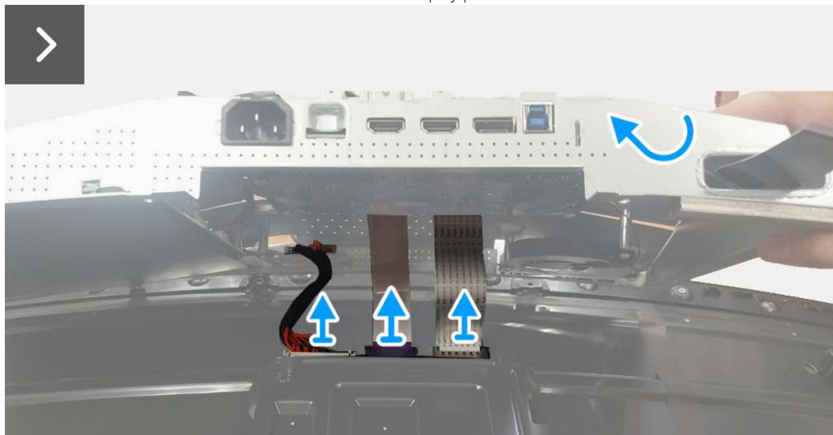
Figure 21. Removing the metal shield
