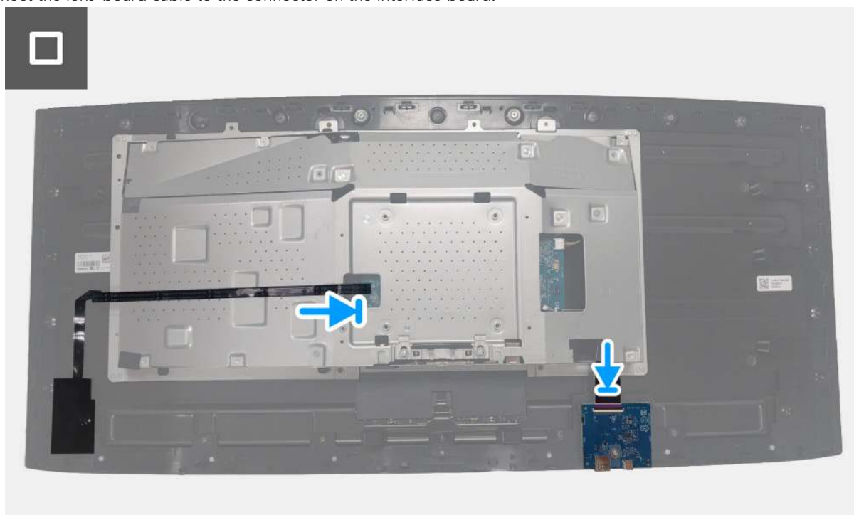
Figure 25. Installing the metal shield
