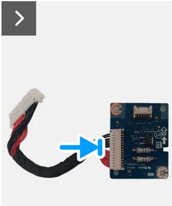
Figure 36. Installing the DC-DC board
