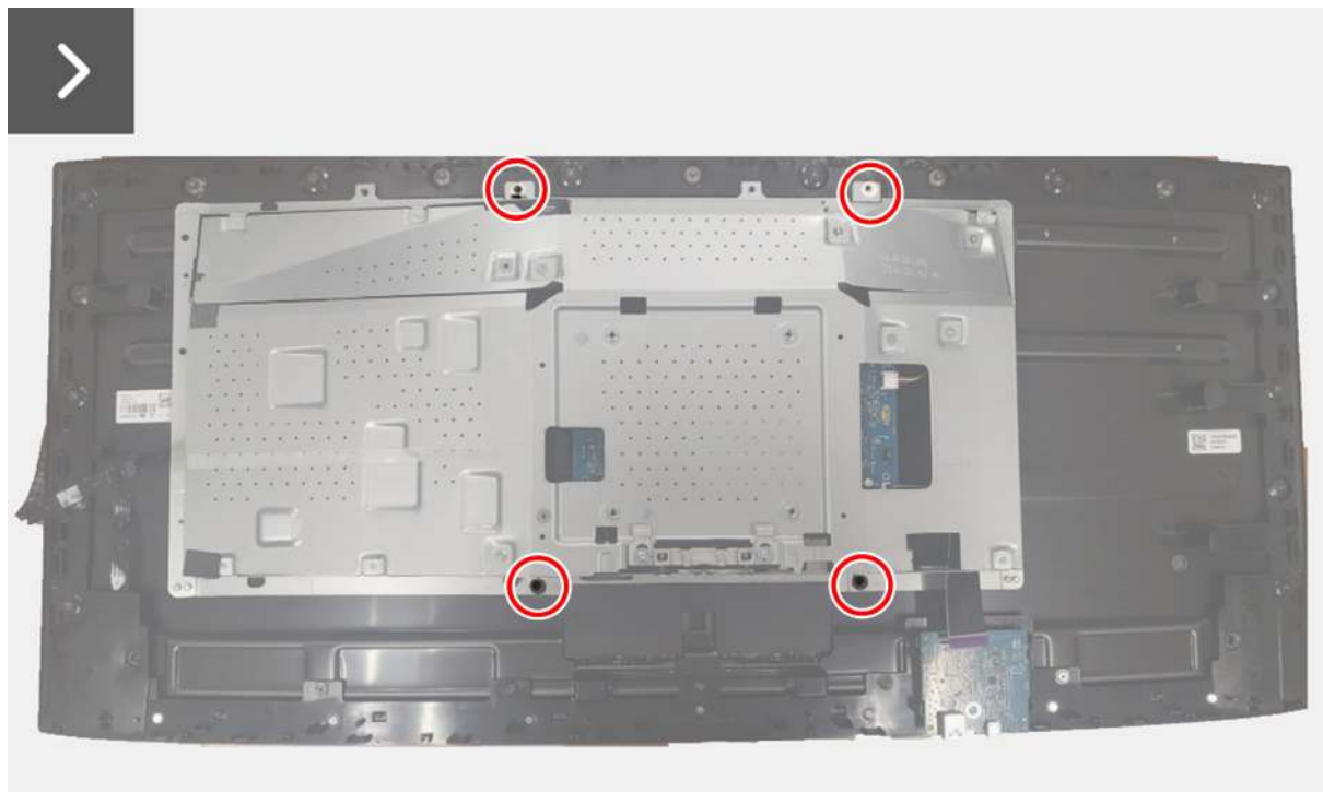
Figure 20. Removing the metal shield
