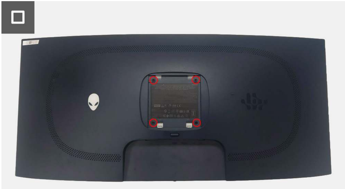
Figure 18. Installing the back cover
