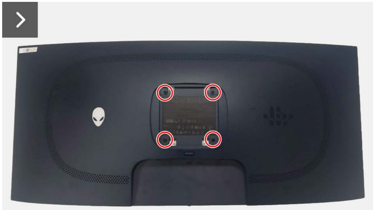
Figure 13. Removing the back cover
