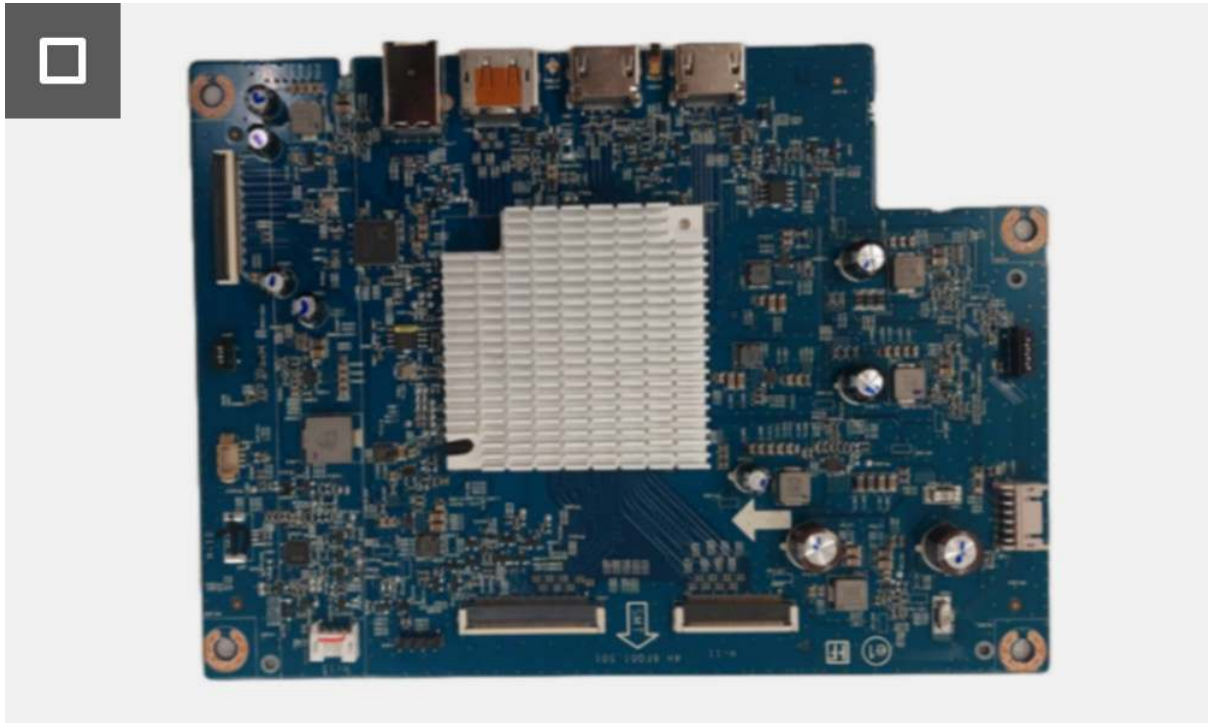
Figure 29. Removing the interface board
