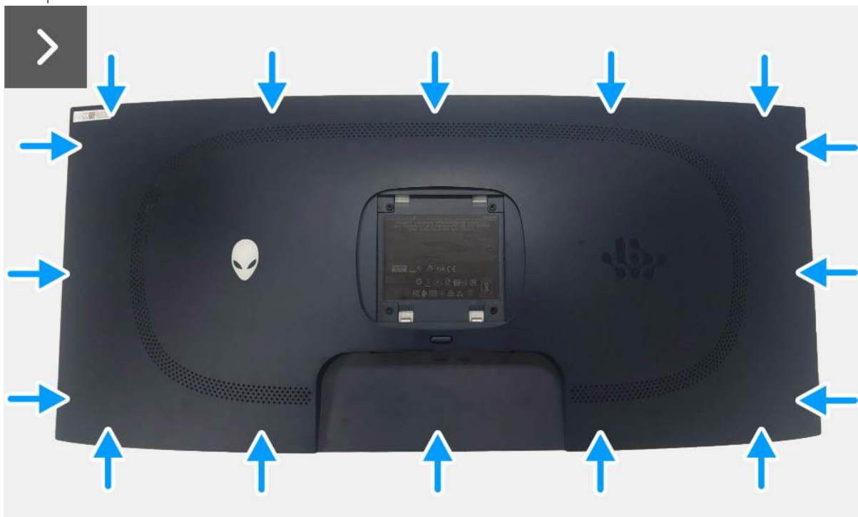
Figure 17. Installing the back cover
