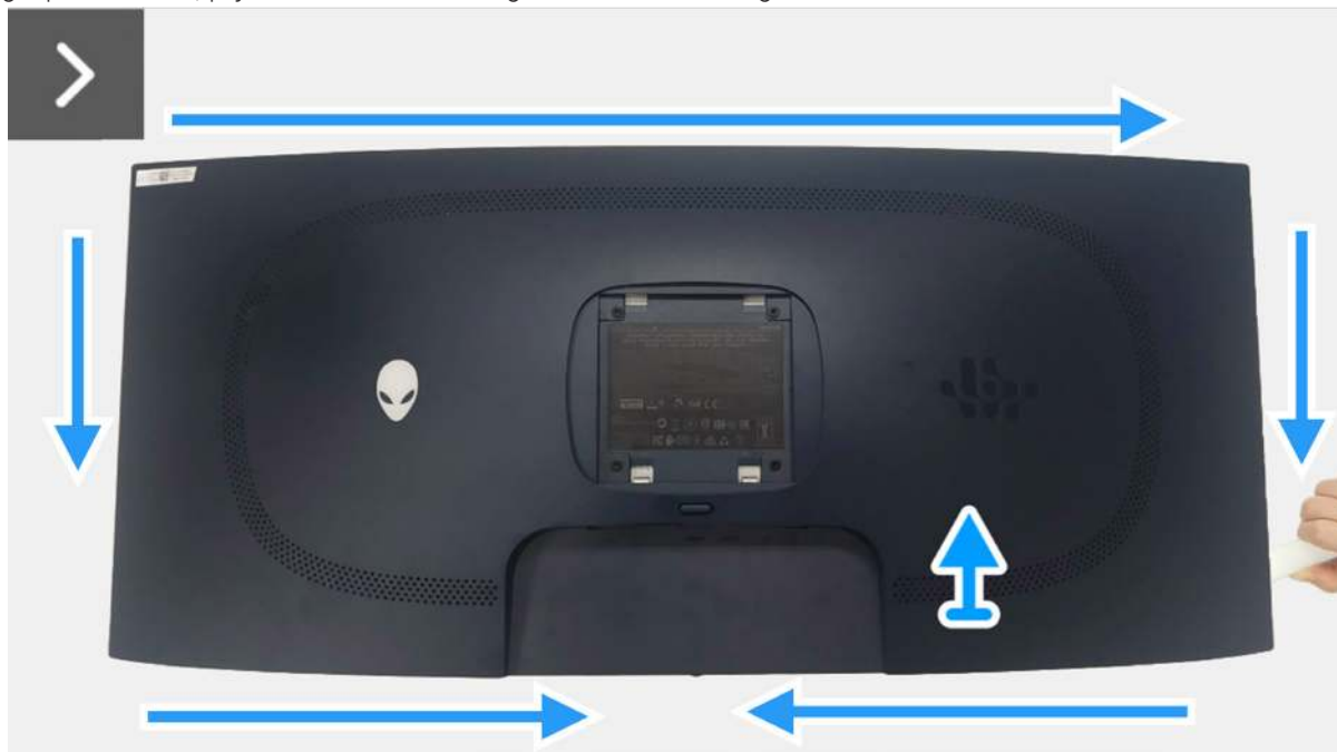
Figure 14. Removing the back cover
