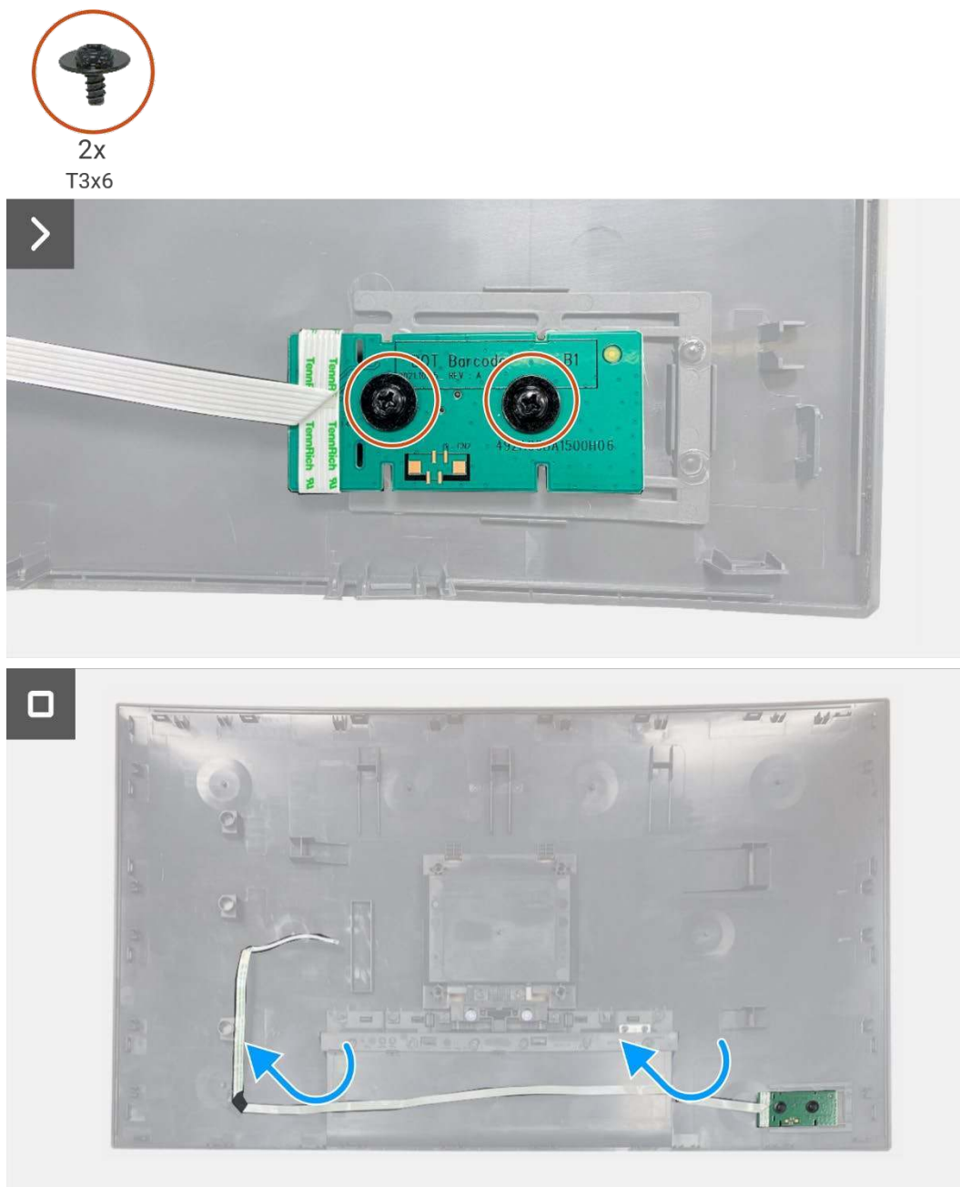
Figure 56. Removing the keypad board
