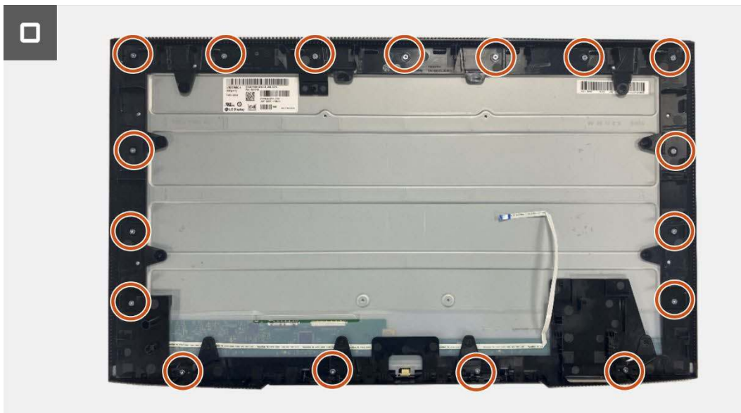
Figure 77. Installing the LED board
