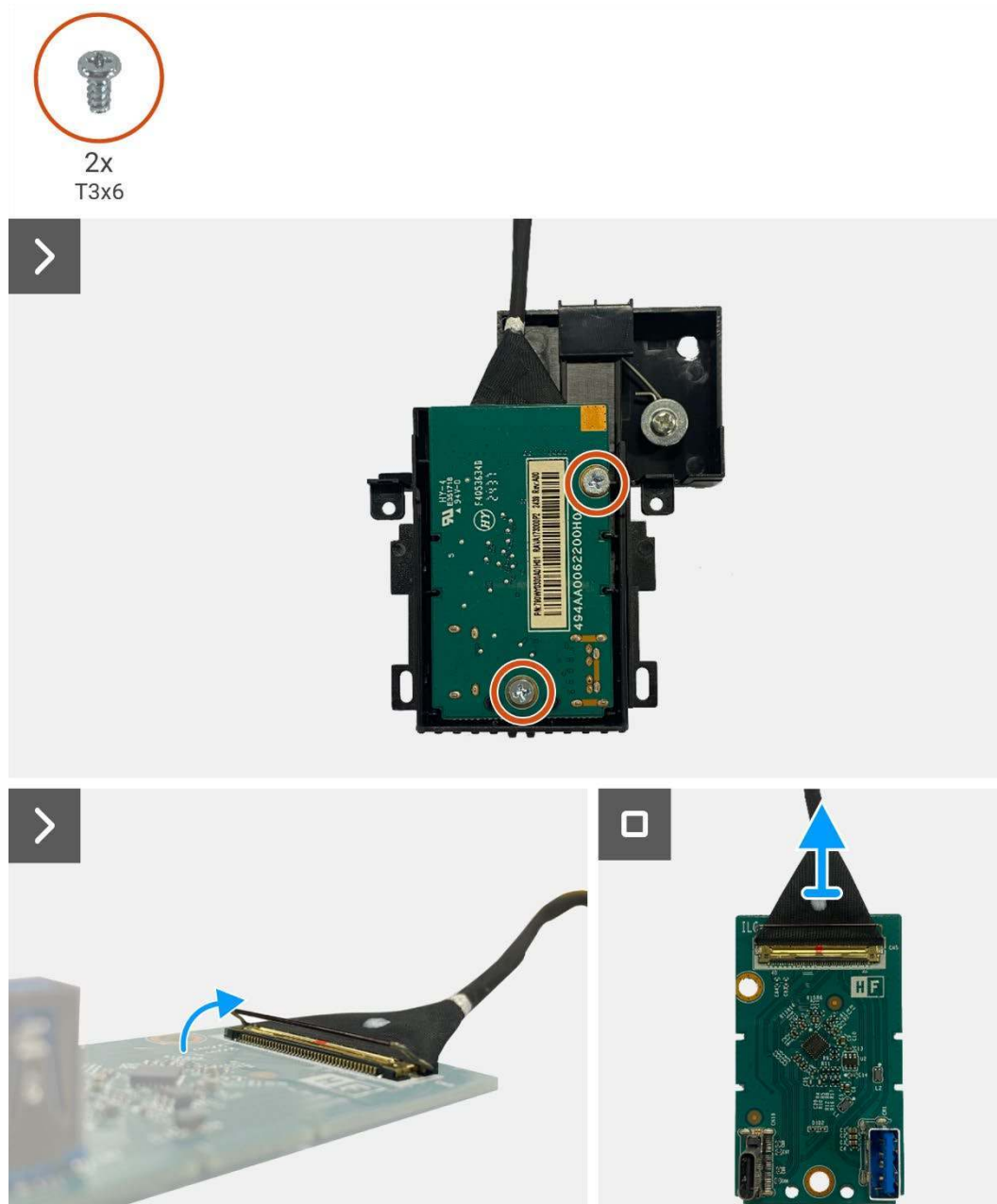
Figure 89. Removing the QAP board
