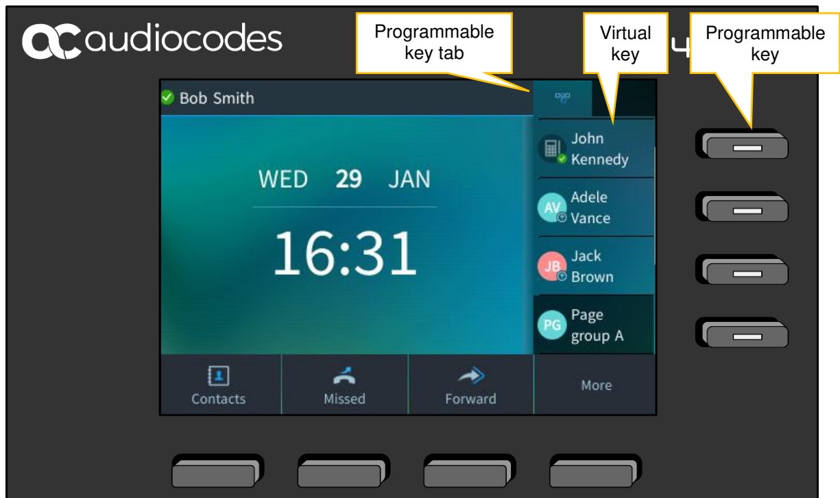
Figure 10: Example of Line-Key, Intercom-Key, Share-Line-Group-Key, and Cloud-paging-Key.
