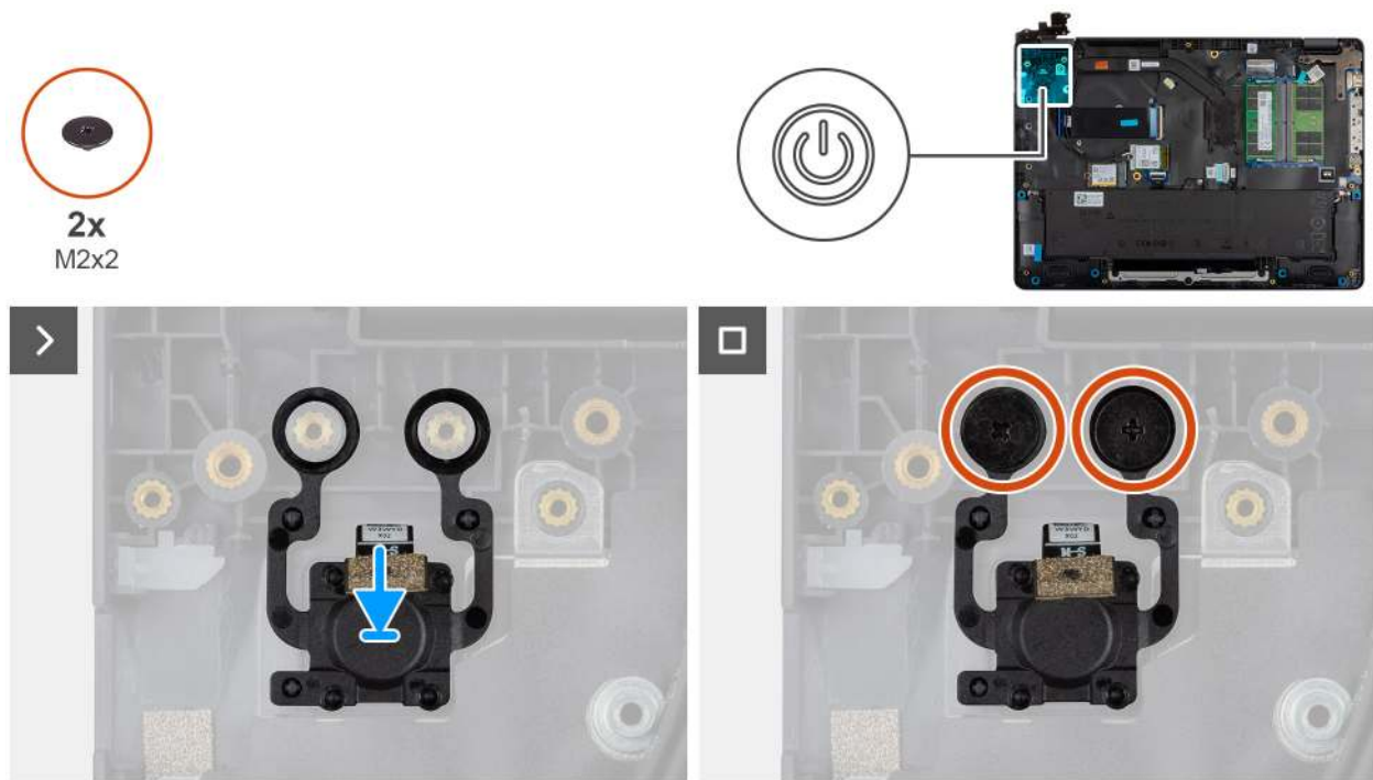
Figure 45. Installing the power button with a fingerprint reader
