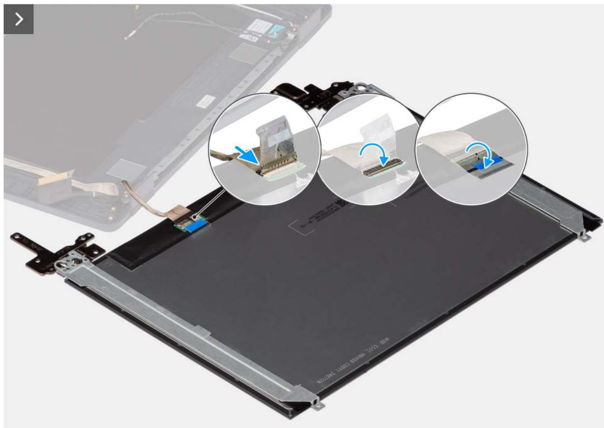
Figure 89. Installing the display-panel assembly
