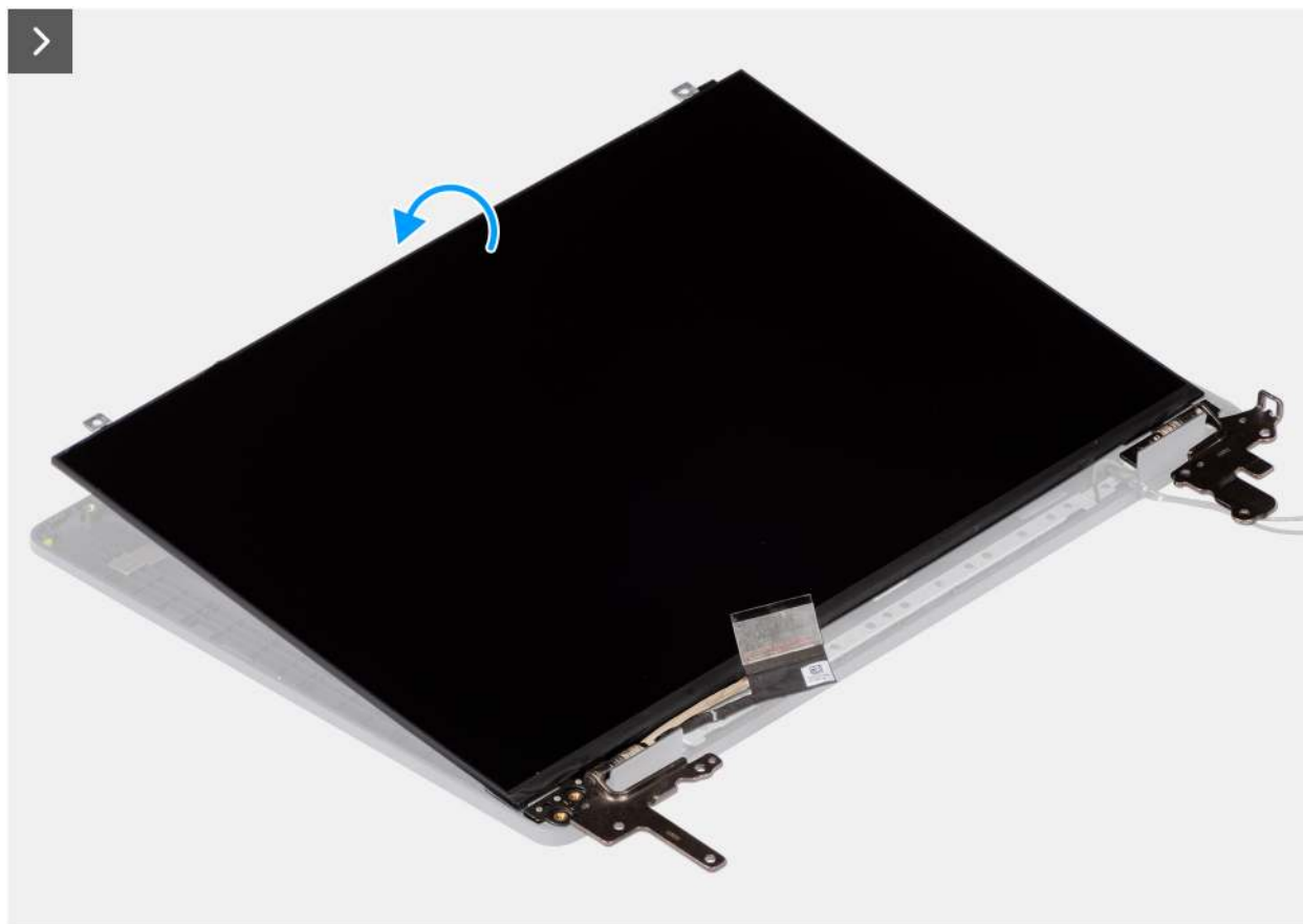
Figure 90. Installing the display-panel assembly
