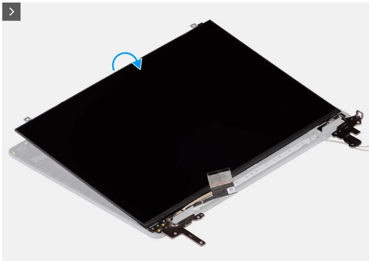
Figure 85. Removing the display-panel assembly
