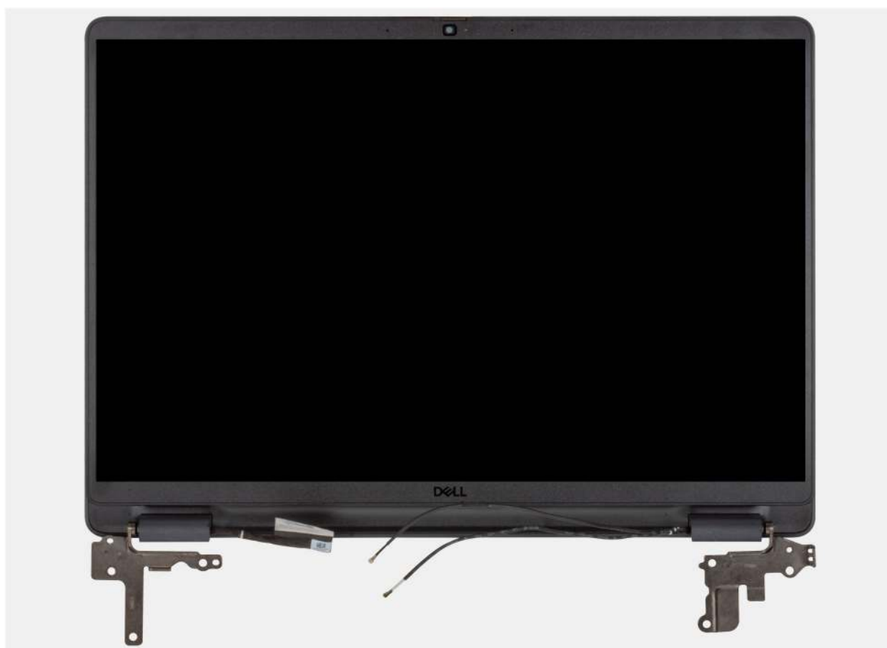
Figure 74. Removing the display assembly
