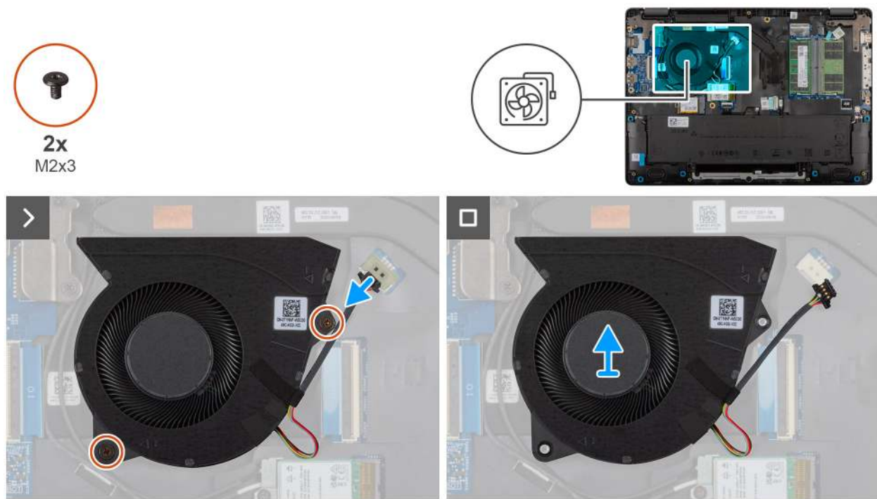
Figure 30. Removing the fan
