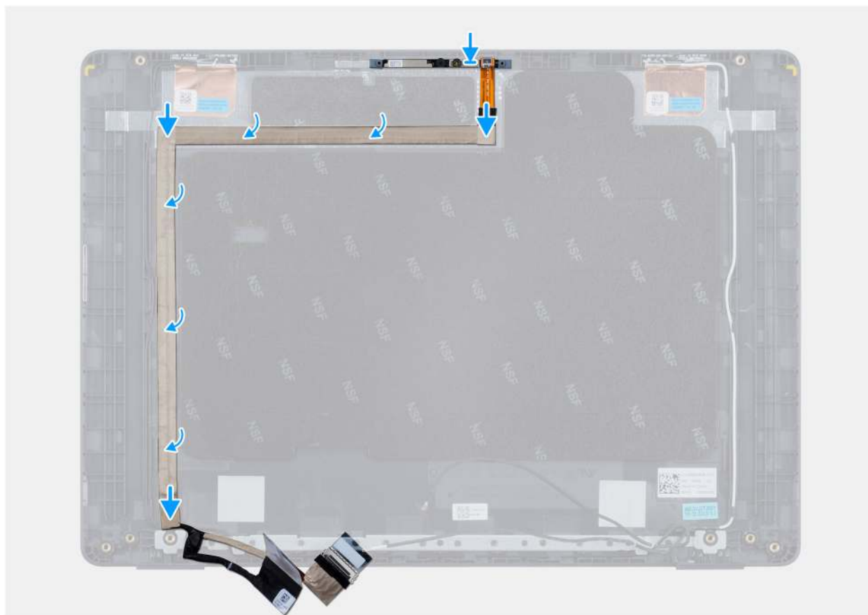
Figure 95. Installing the eDP cable
