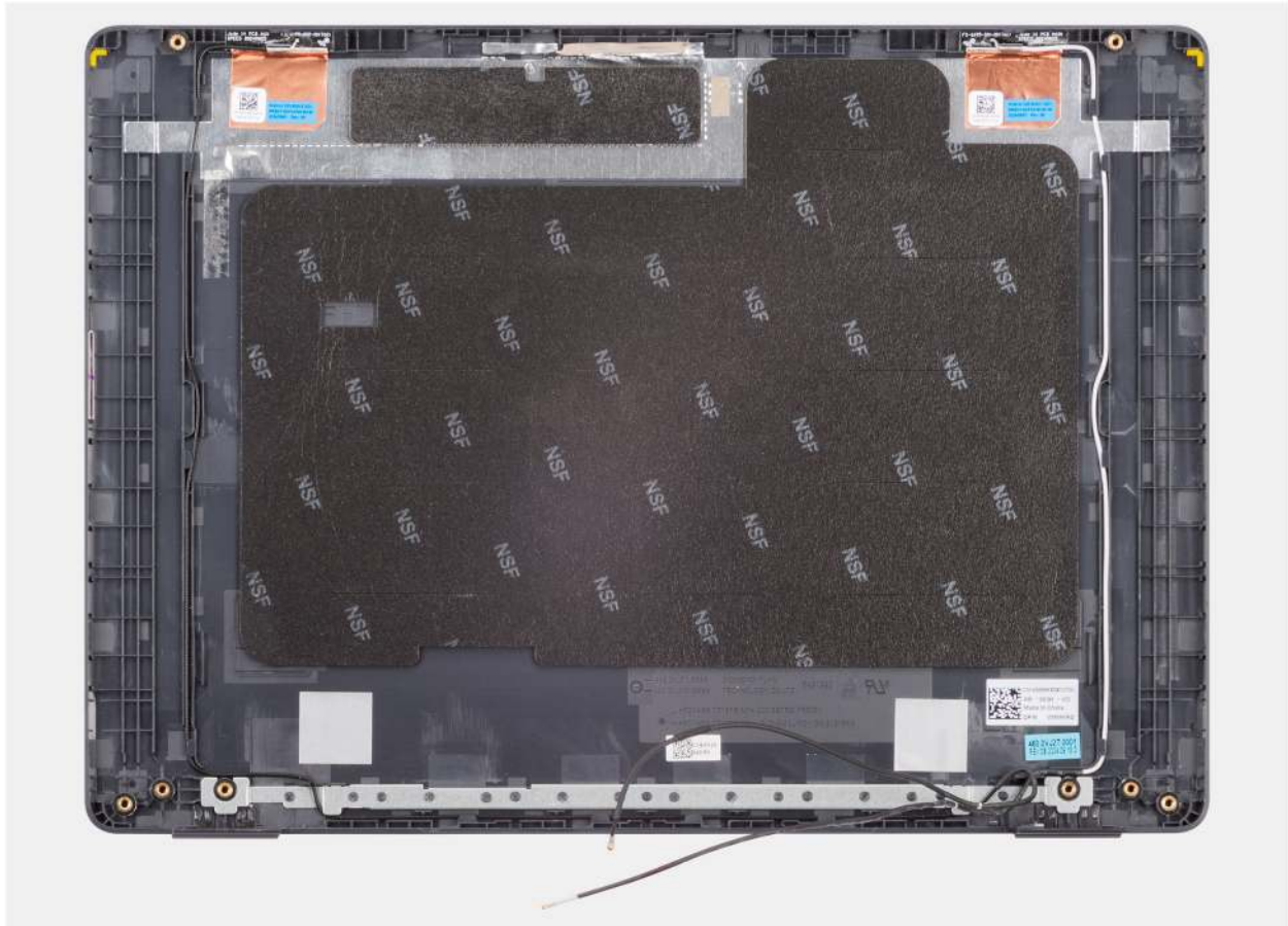
Figure 96. Removing the display back-cover assembly
