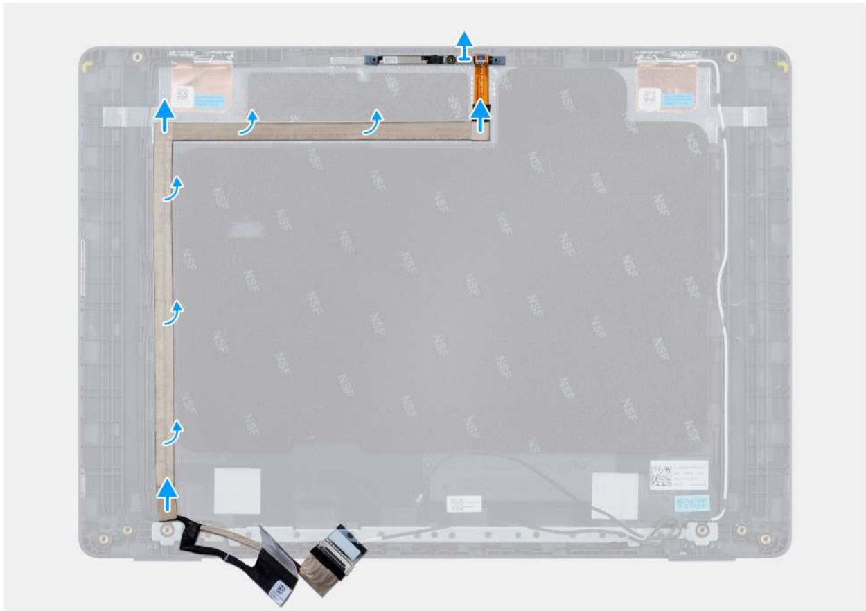
Figure 94. Removing the eDP cable
