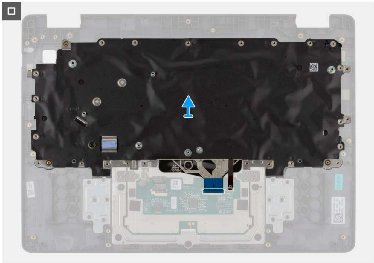
Figure 61. Removing the keyboard
