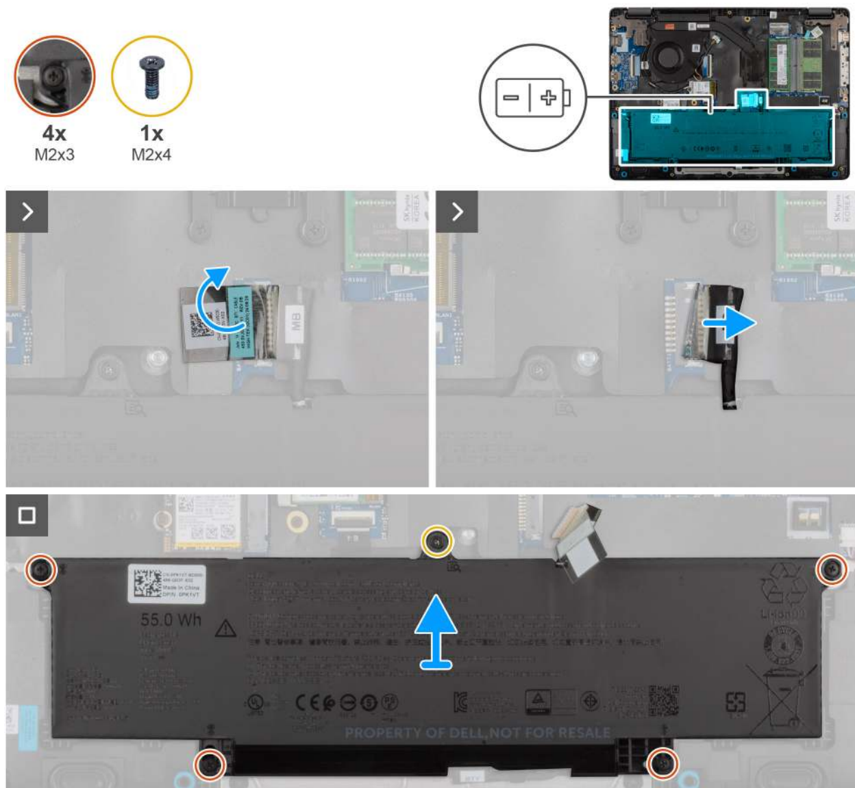
Figure 17. Removing the battery
