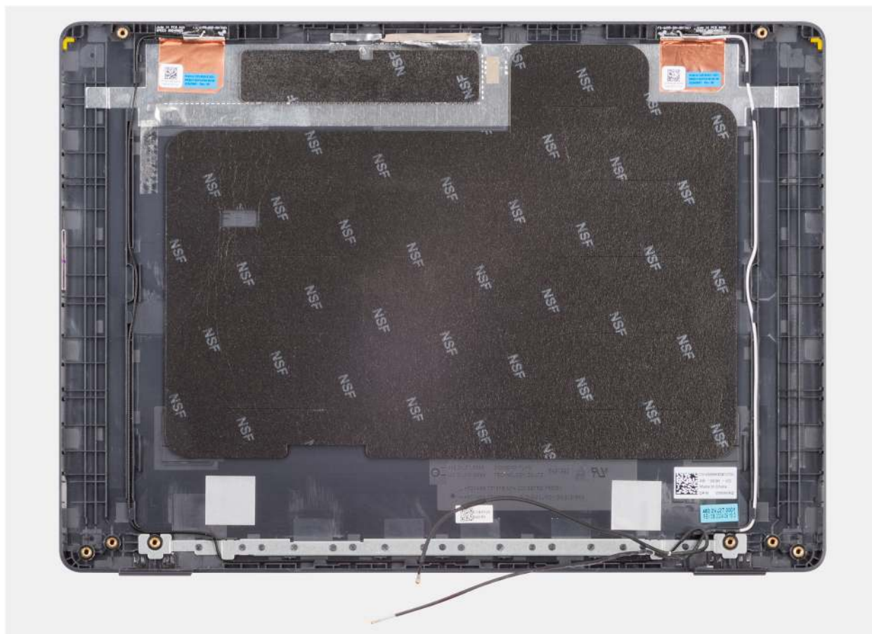
Figure 97. Installing the display back-cover assembly
