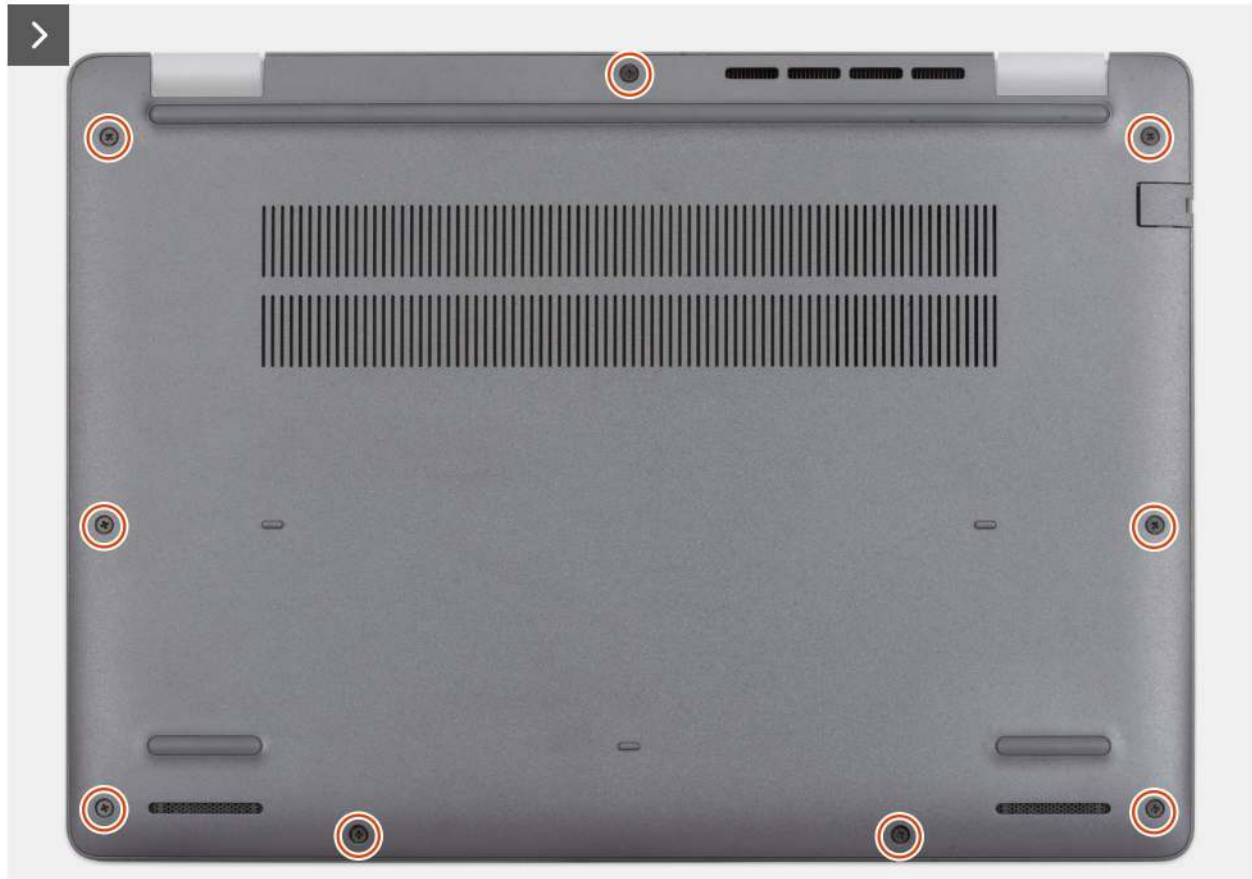
Figure 11. Removing the base cover
