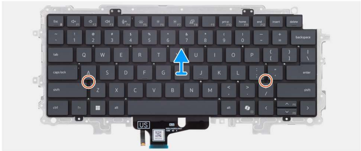
Figure 66. Removing the keyboard support plate
