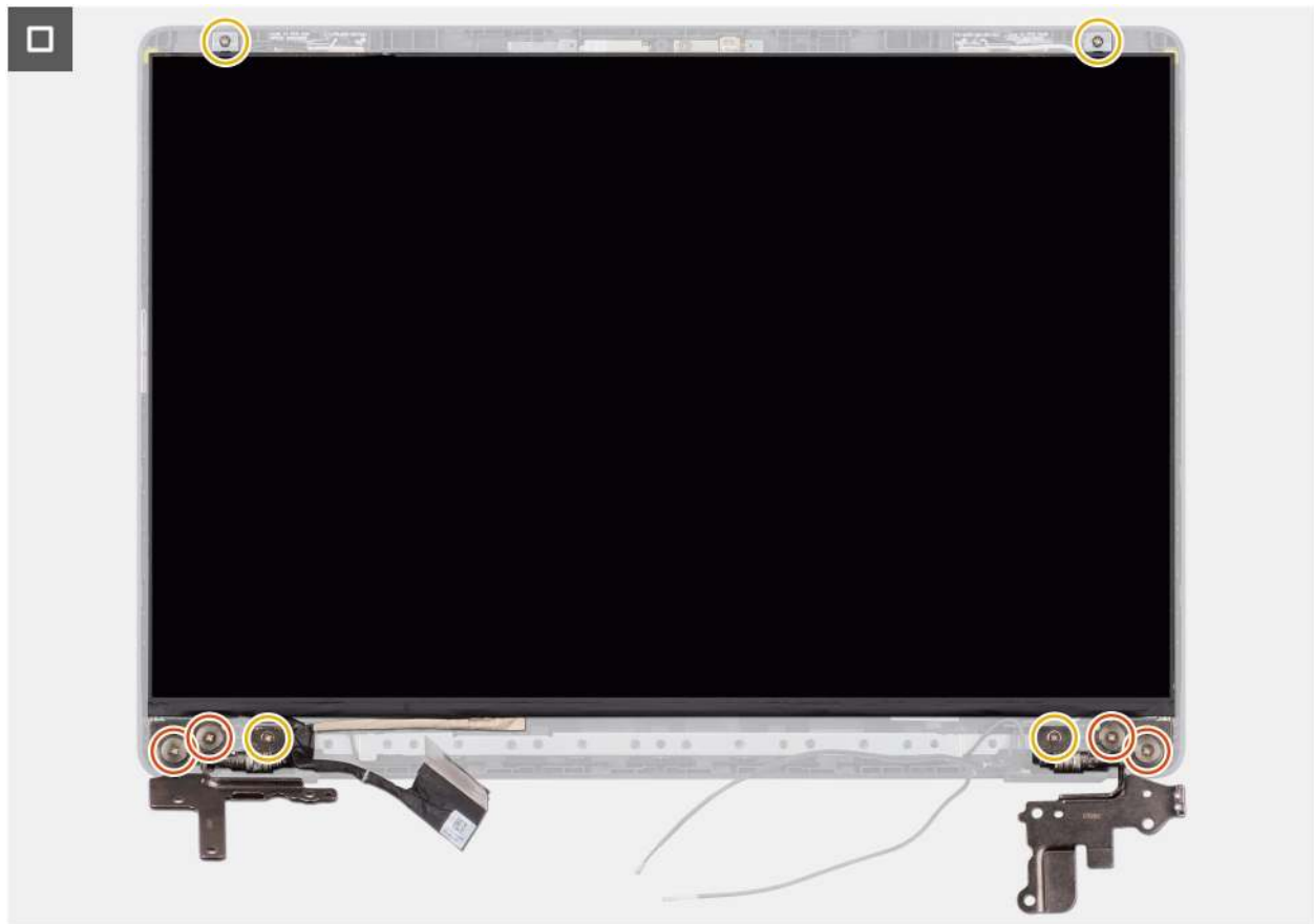
Figure 91. Installing the display-panel assembly
