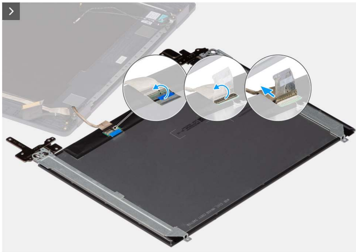
Figure 86. Removing the display-panel assembly
