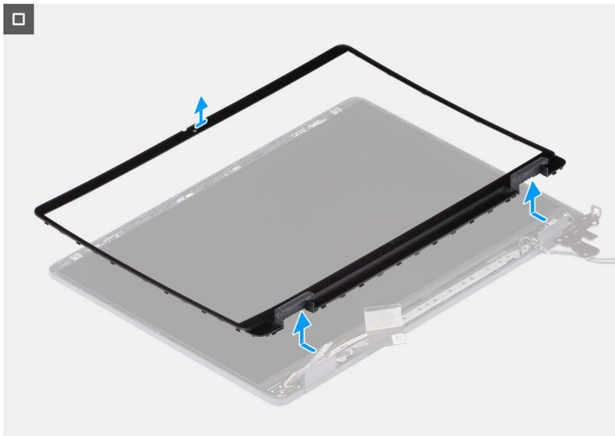
Figure 81. Removing the display bezel
