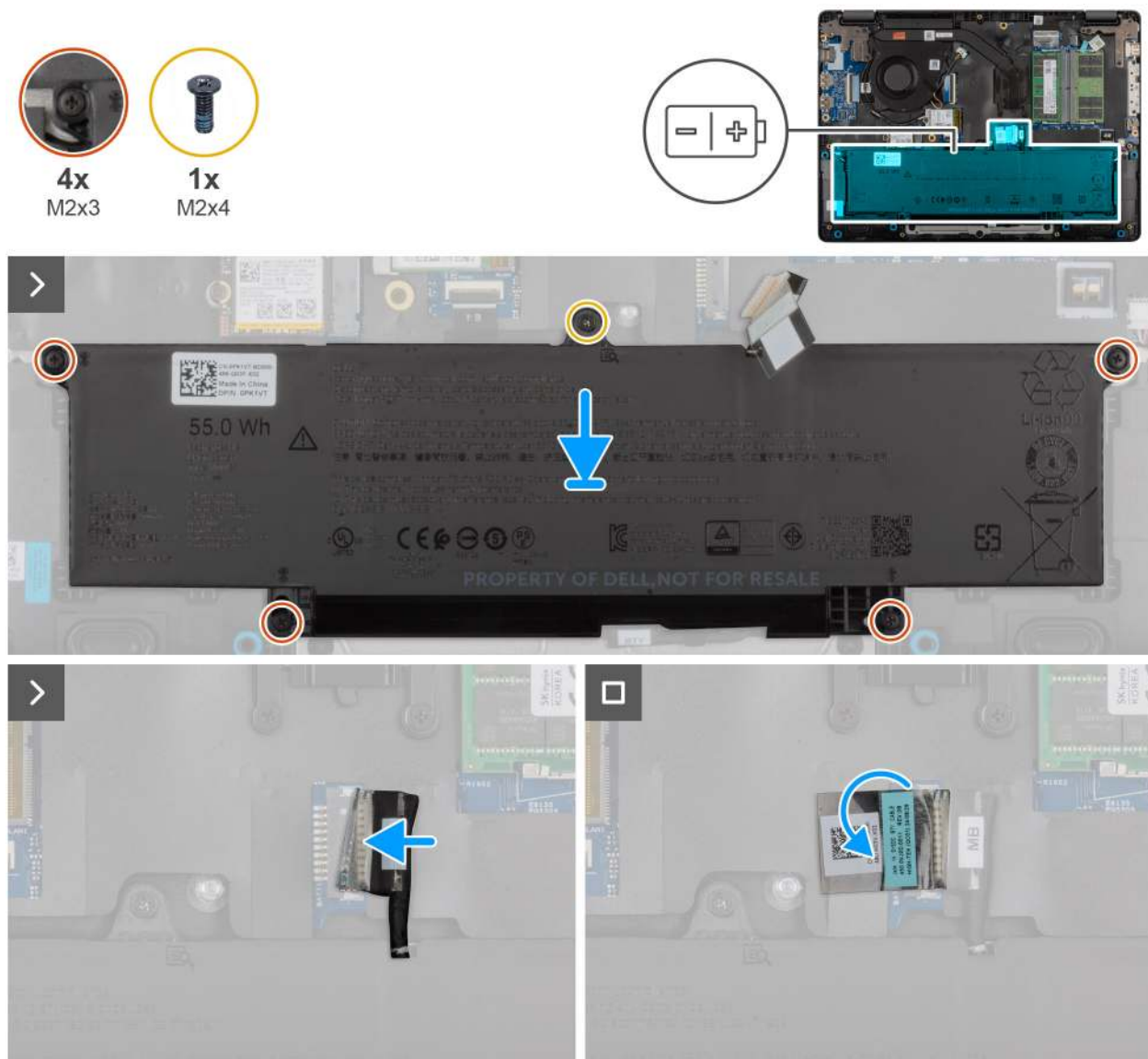
Figure 18. Installing the battery
