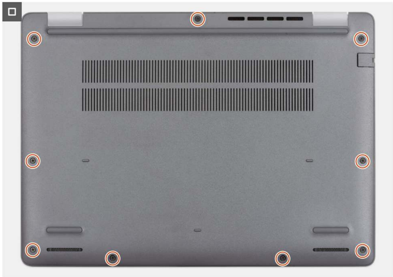
Figure 16. Installing the base cover
