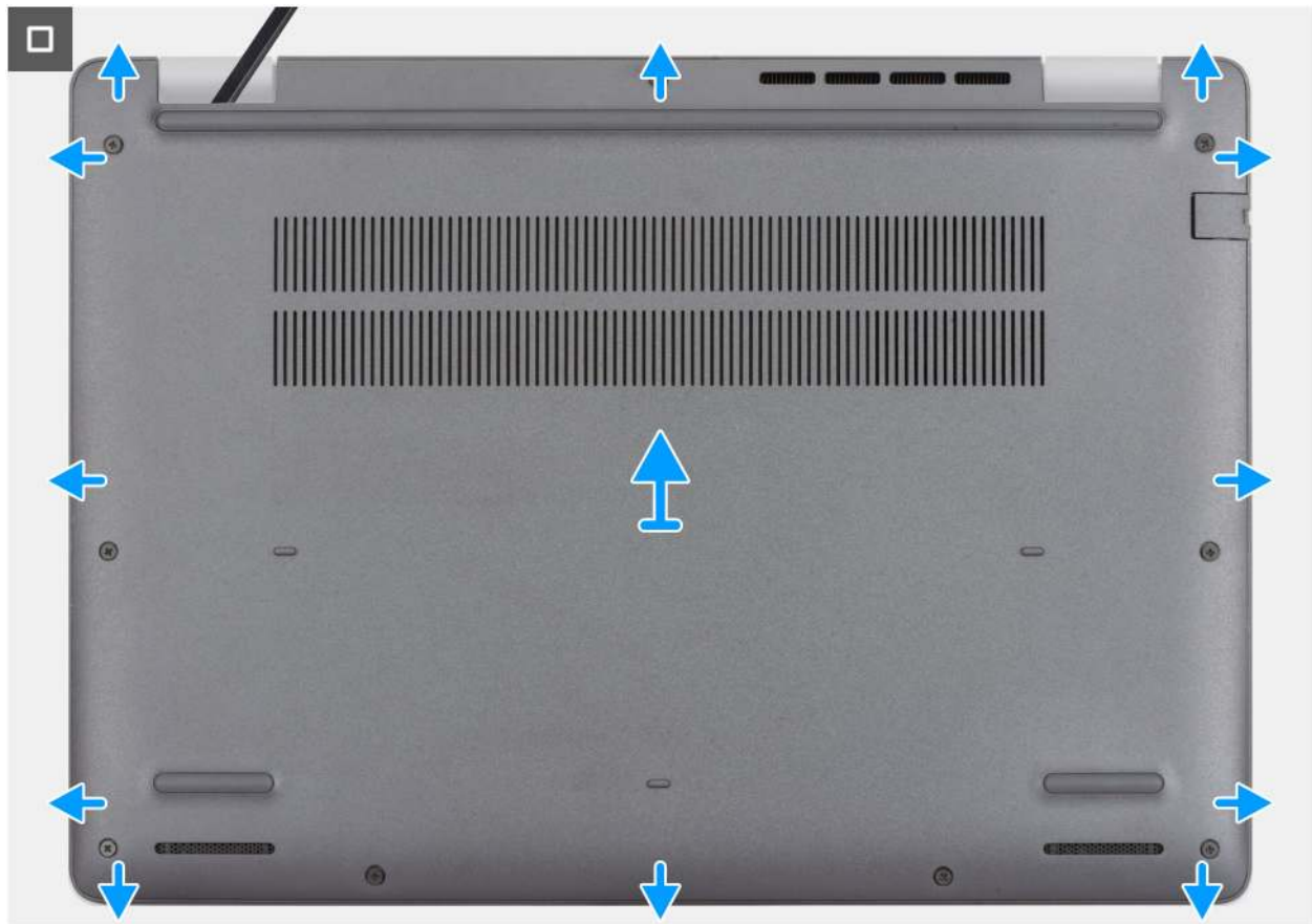
Figure 12. Removing the base cover
