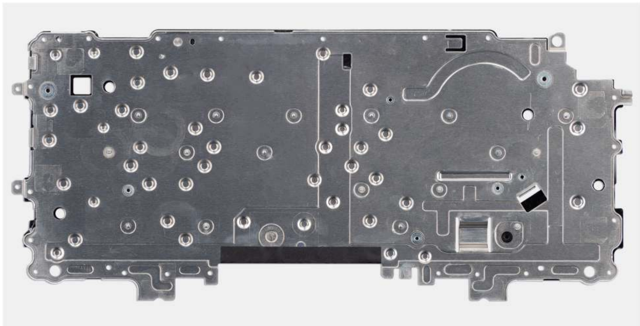
Figure 67. Removing the keyboard support plate
