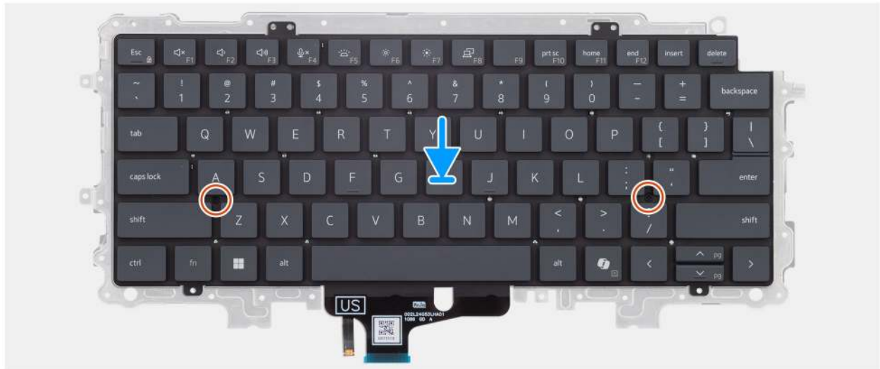
Figure 69. Installing the keyboard support plate
