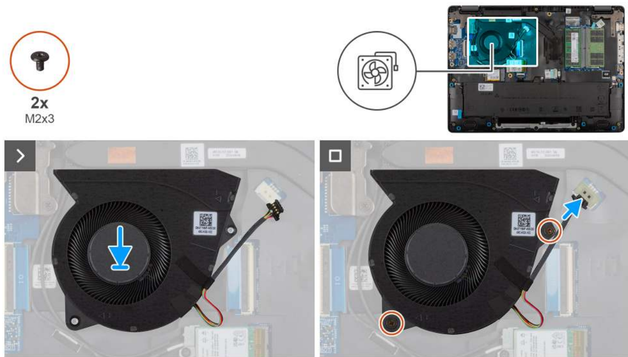
Figure 31. Installing the fan
