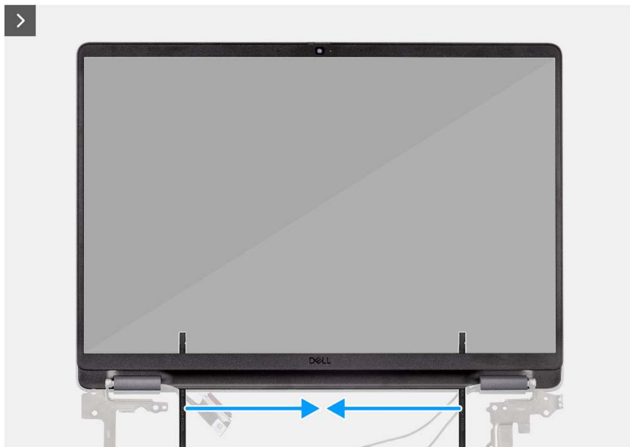
Figure 78. Removing the display bezel
