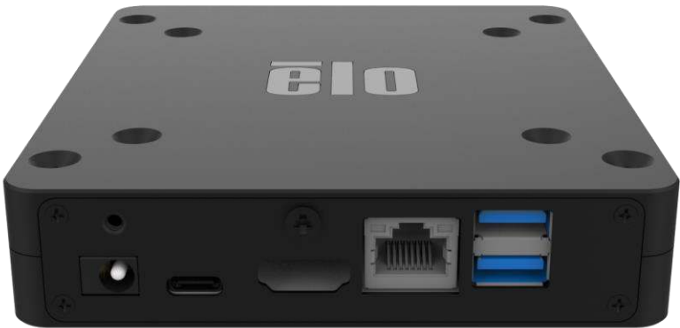
DC In Type C HDMI Ethernet USB 3.0
