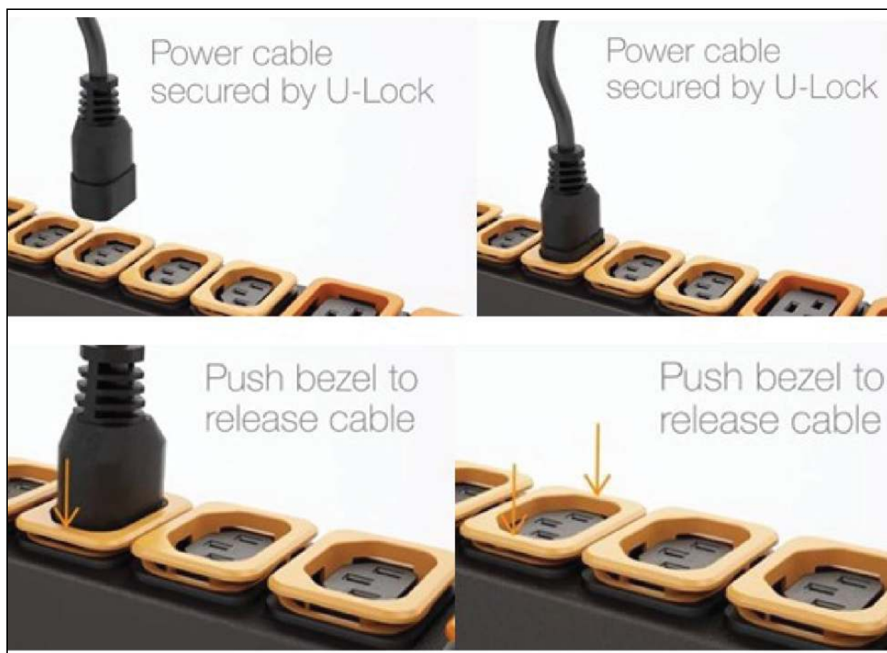
Figure 3.15 U-Lock Cord Retention Operation
