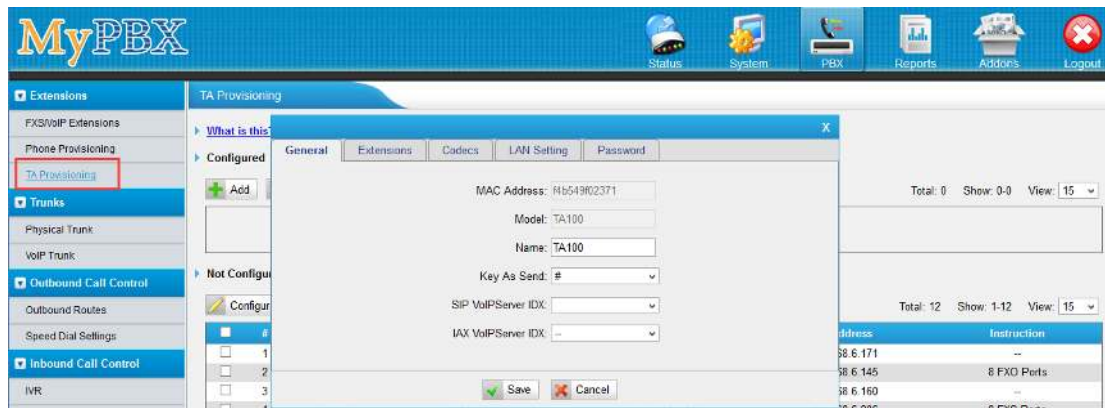
Figure 11-4 MyPBX TA Provisioning
