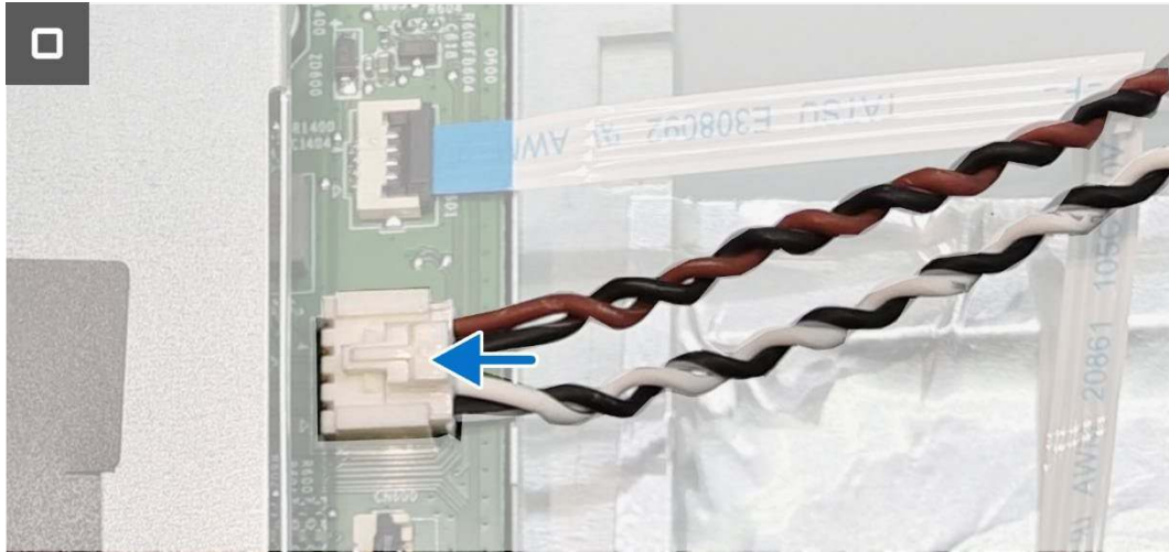
Figure 27. Installing the speakers
