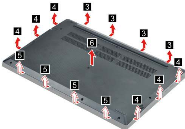
Figure 106. Pry up the latches and remove the lower case
