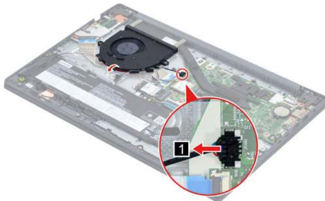
Figure 85. Disconnect the fan cable from the system board
