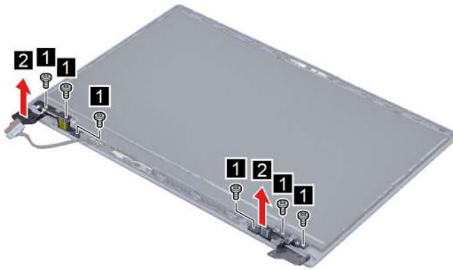
Figure 34. Remove six screws and then remove the hinges
