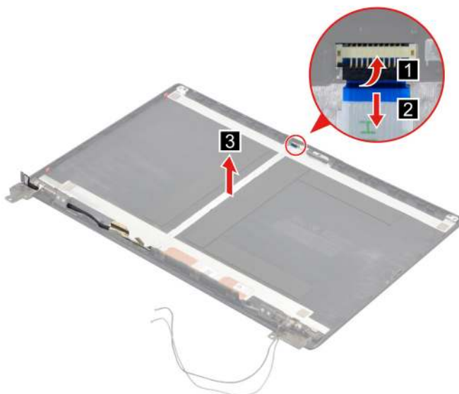
Figure 74. Disconnect the EDP cable from the camera board and then remove the EDP cable
