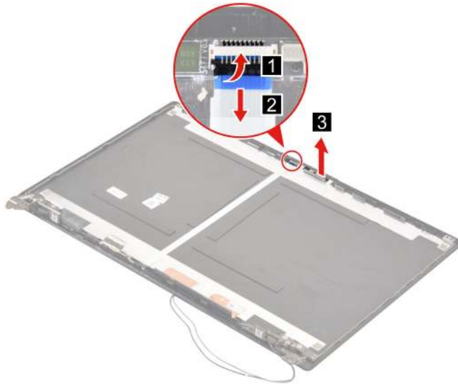
Figure 139. Disconnect the EDP cable from the camera board and then remove the camera
