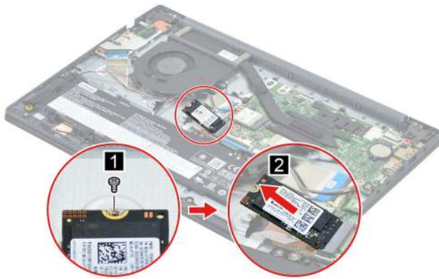
Figure 81. Remove one screw then remove the SSD by pulling it away from the slot
