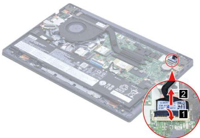
Figure 31. Disconnect the EDP cable from the system board
