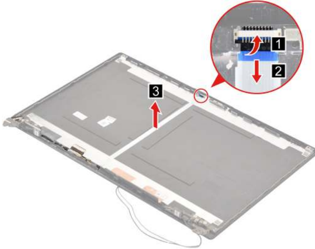
Figure 138. Disconnect the EDP cable from the camera board and then remove the EDP cable
