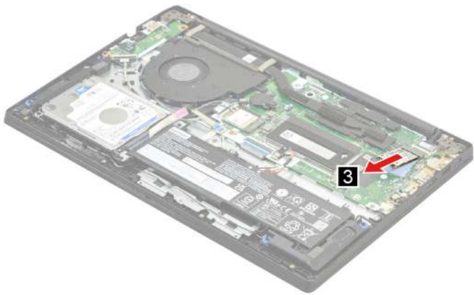
Figure 115. Remove the SSD by pulling it away from the slot
