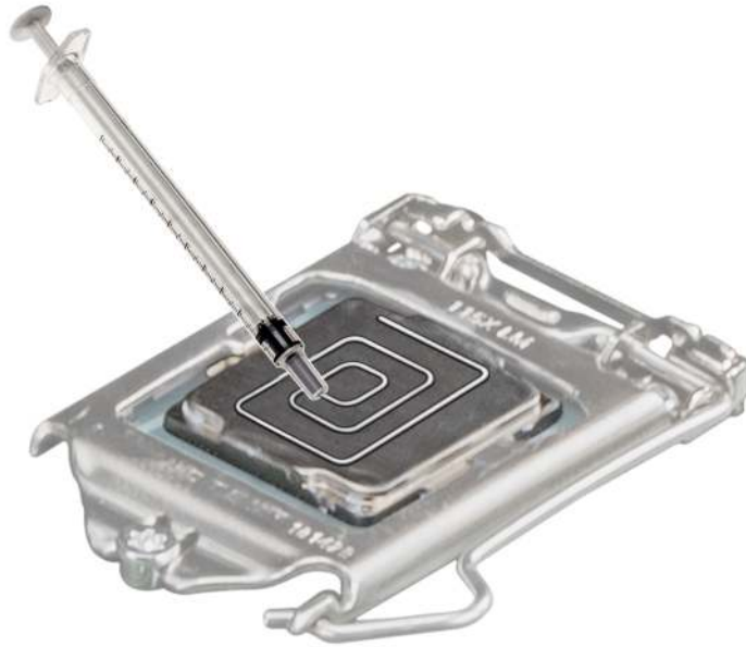
Figure 42. Applying thermal grease on top of the processor
