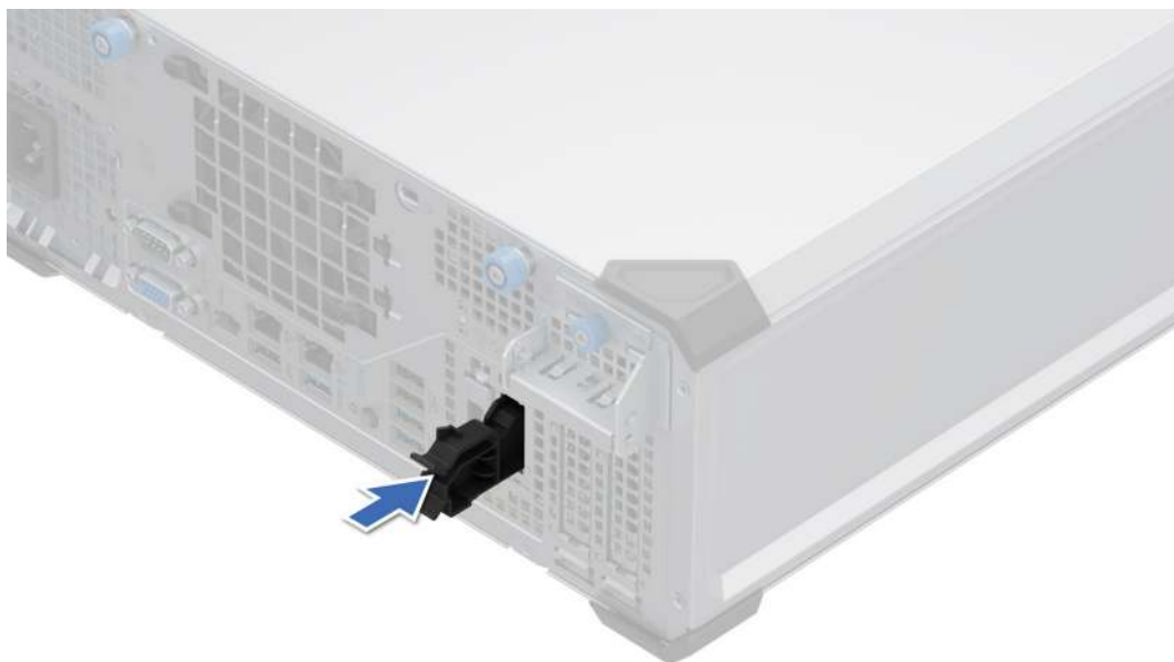
Figure 55. Installing the BOSS-N1 card carrier blank
