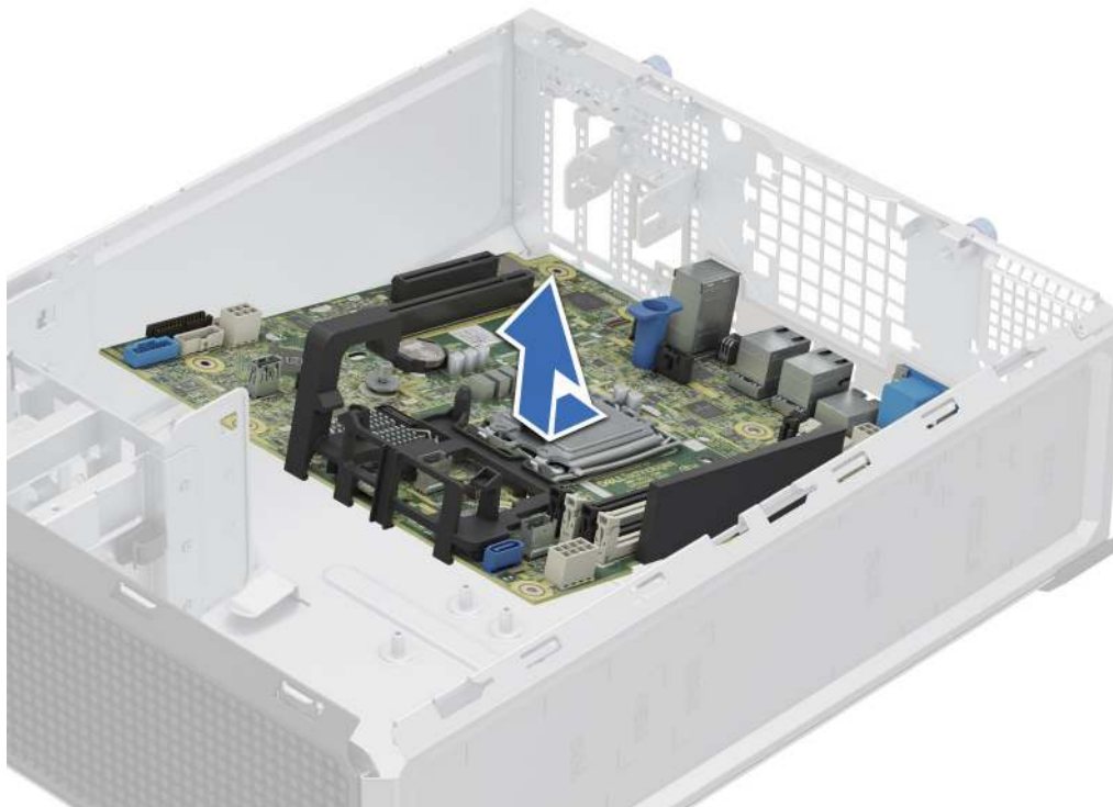
Figure 64. Removing the system board
