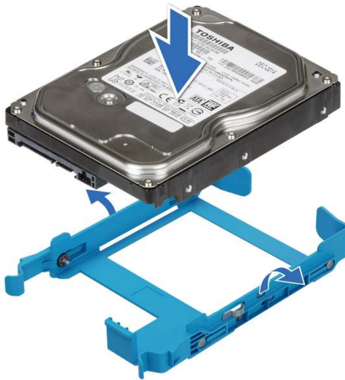
Figure 27. Installing a drive into the drive carrier
