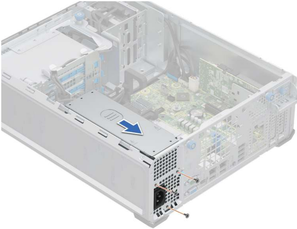
Figure 60. Installing the cabled PSU
