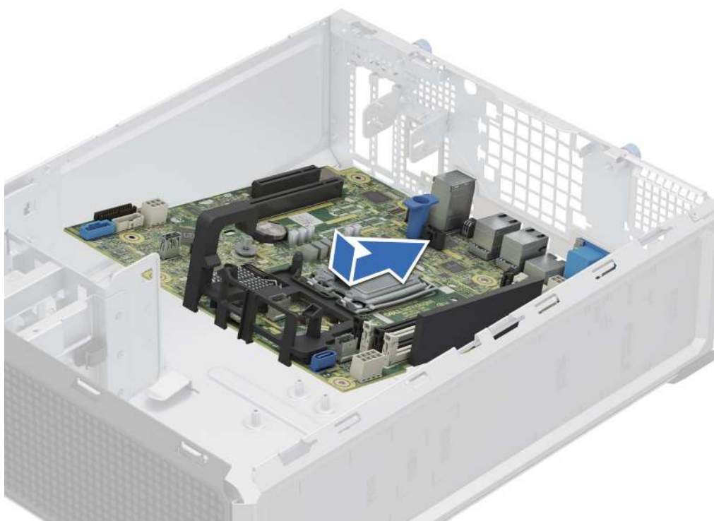
Figure 65. Installing the system board
