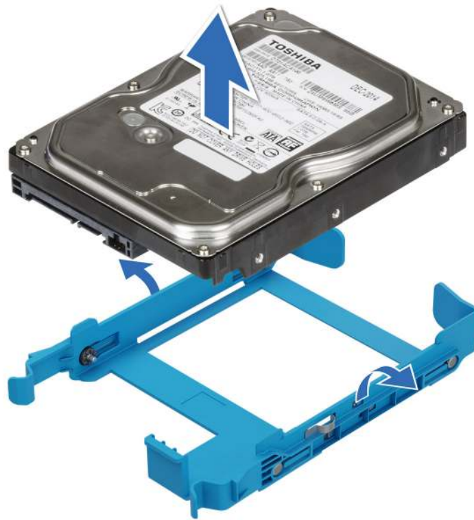
Figure 26. Removing the drive from the drive carrier
