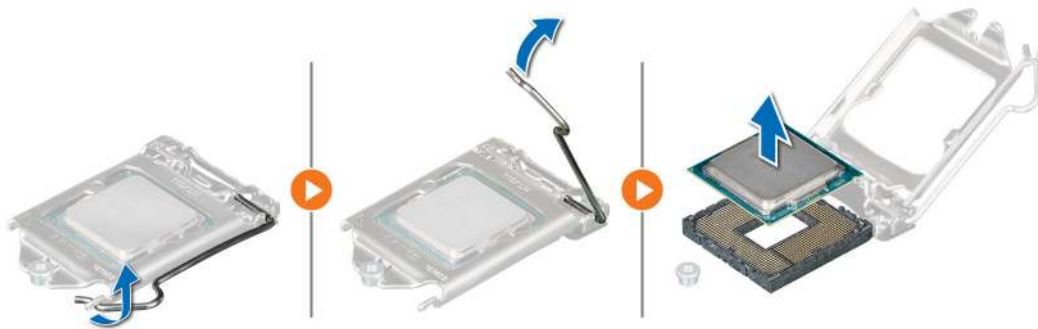
Figure 40. Removing the processor
