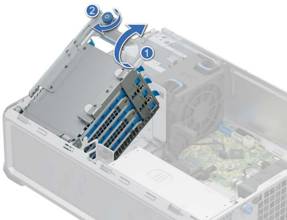
Figure 24. Installing a drive carrier
