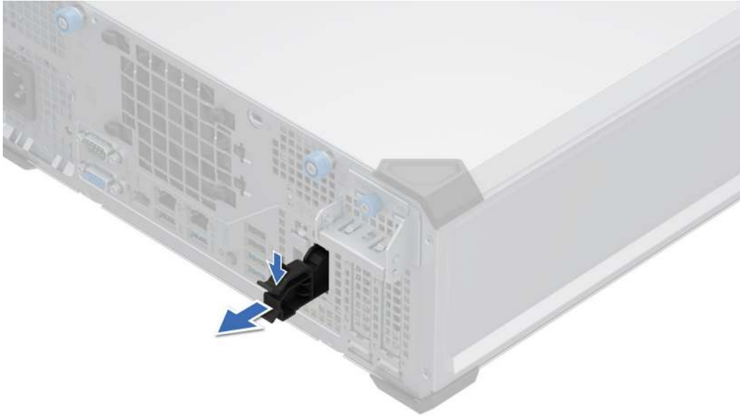
Figure 51. Removing the BOSS-N1 module blank
