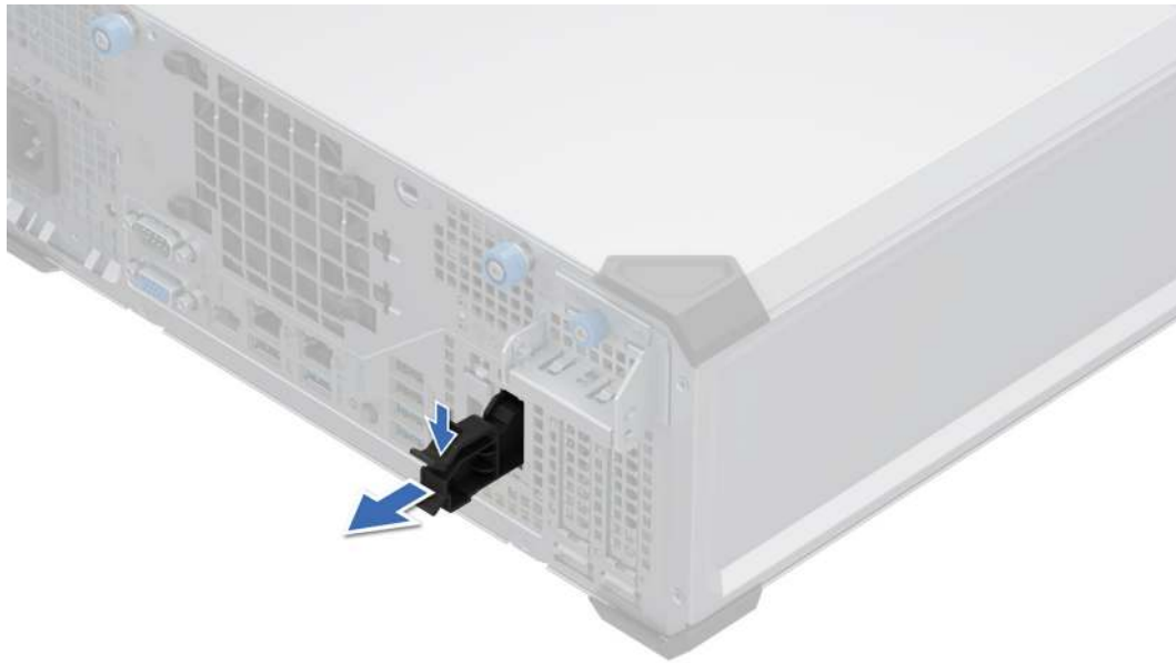
Figure 56. Removing the BOSS-N1 card carrier blank
