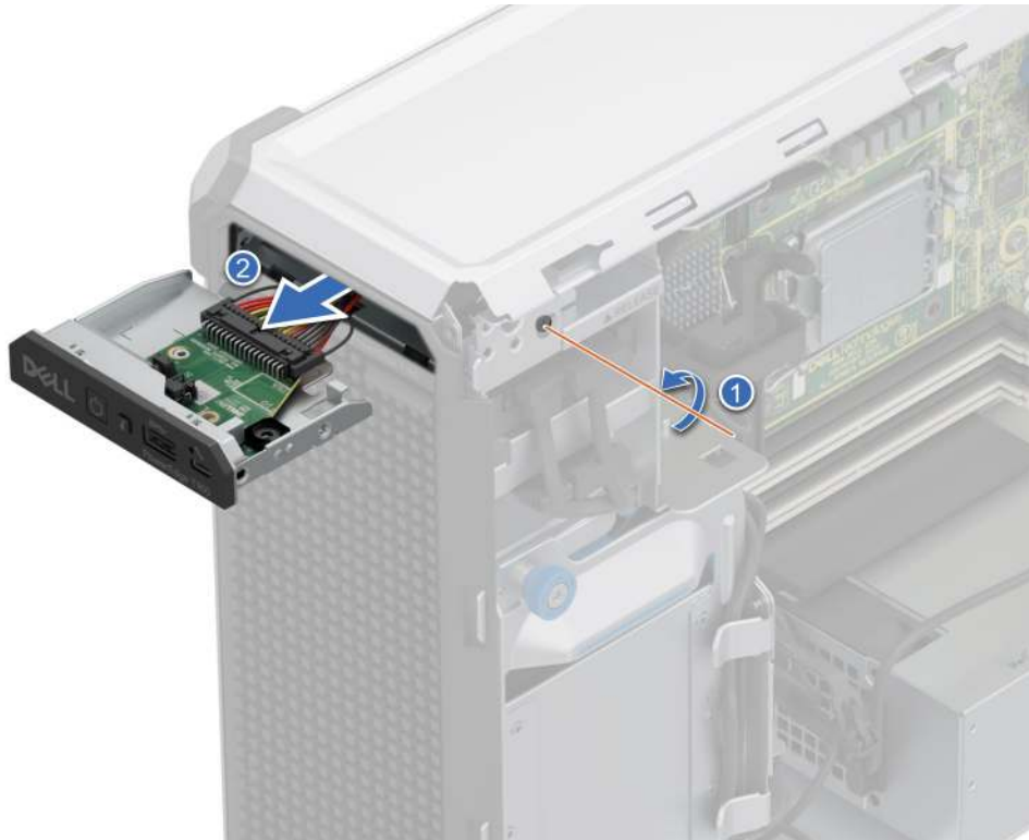
Figure 68. Removing the control panel cage
