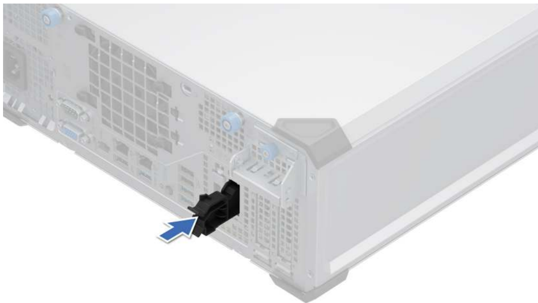
Figure 50. Installing the BOSS-N1 module blank
