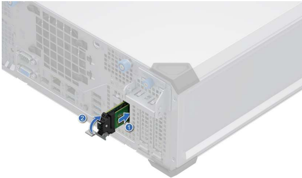
Figure 58. Installing the BOSS-N1 card carrier
