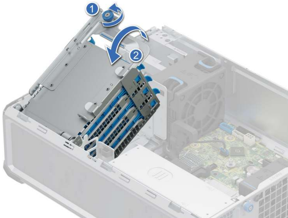
Figure 20. Removing a drive from drive cage
