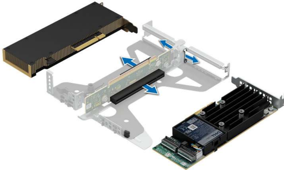
Figure 50. Removing an expansion card from the riser
