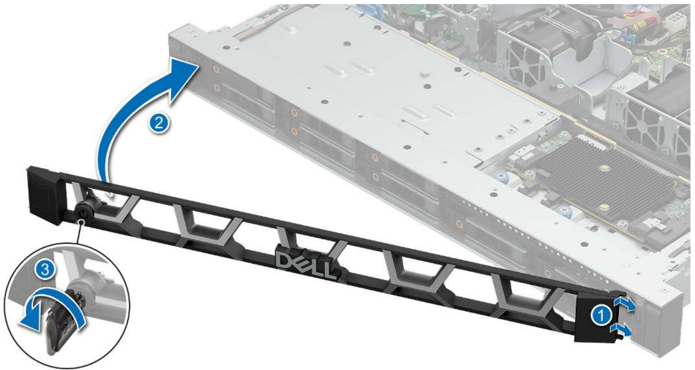
Figure 15. Installing the front bezel
