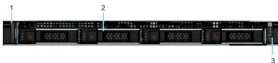
Figure 1. Front view of 4 x 3.5-inch drive system
