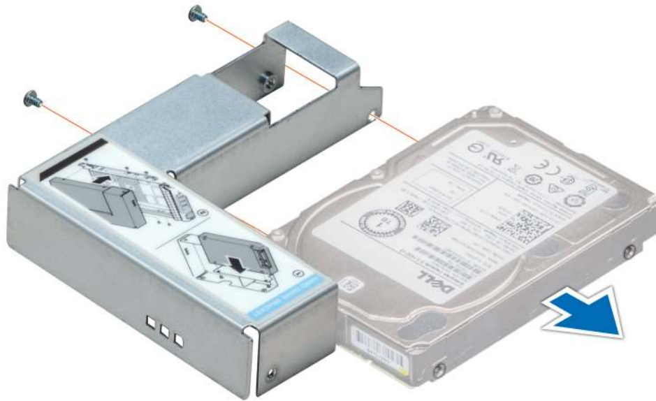
Figure 39. Removing a 2.5 inch drive from a 3.5-inch drive adapter
