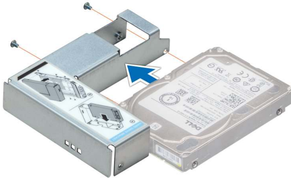
Figure 40. Installing a 2.5-inch drive into a 3.5-inch drive adapter
