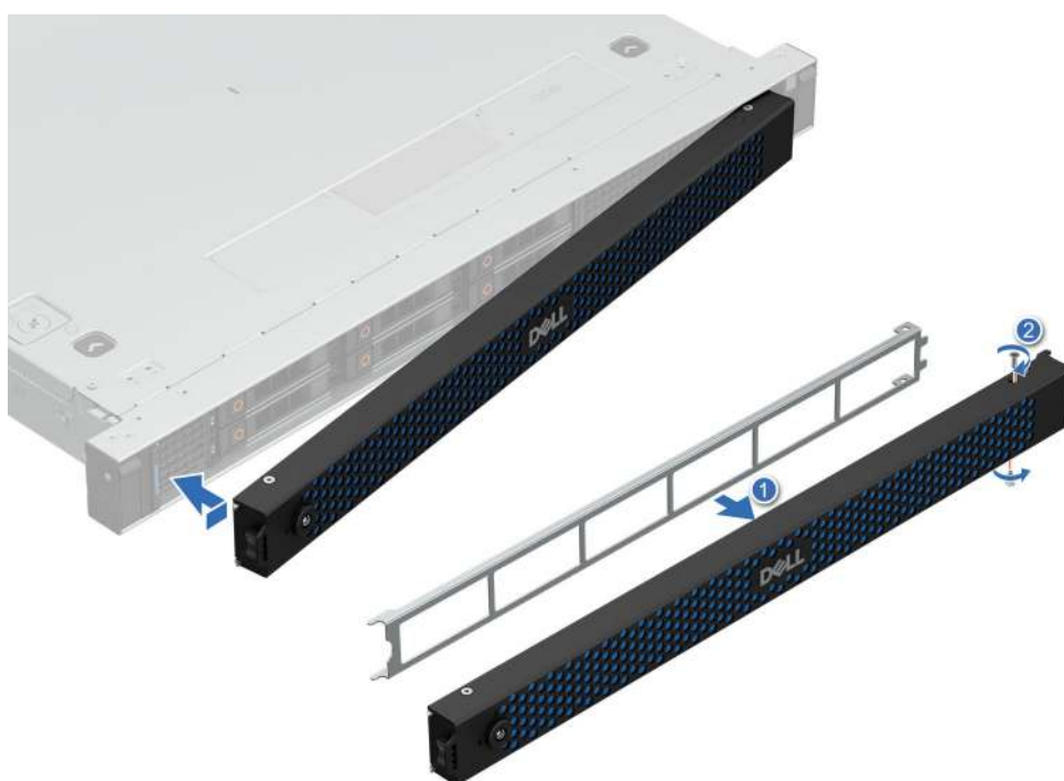
Figure 87. Installing the filter bezel
