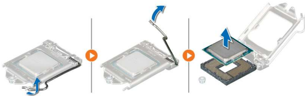
Figure 45. Removing the processor
