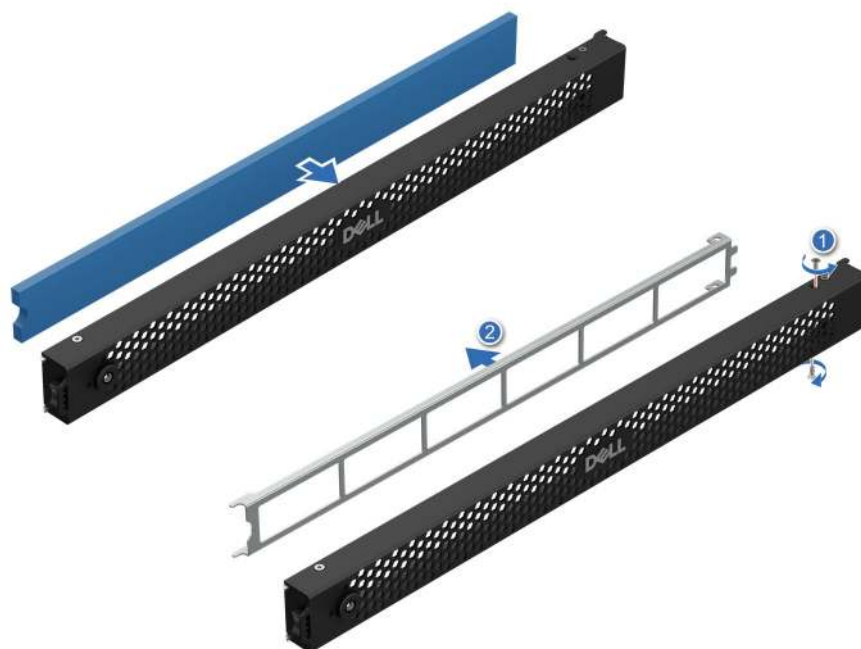
Figure 86. Installing the filter
