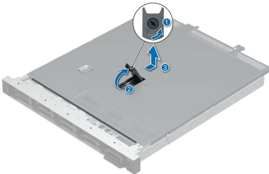
Figure 16. Removing the system cover
