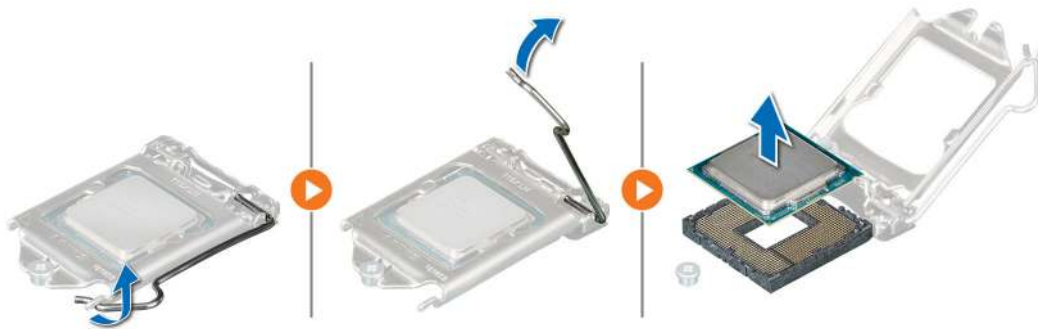
Figure 59. Removing the processor
