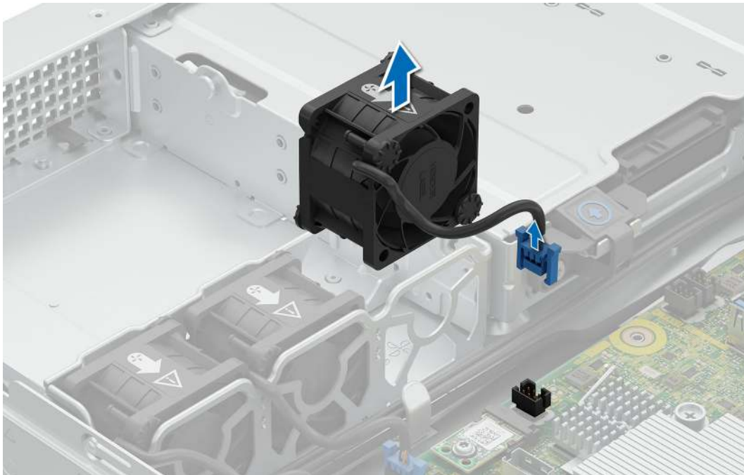
Figure 31. Removing cooling fan
