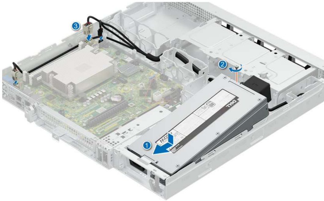
Figure 86. Installing a cabled power supply unit (PSU)
