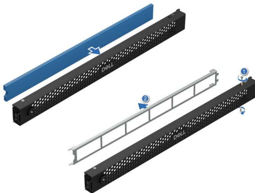
Figure 98. Installing the filter
