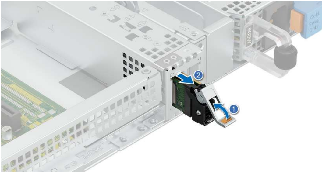
Figure 73. Removing the BOSS-N1 M.2 module
