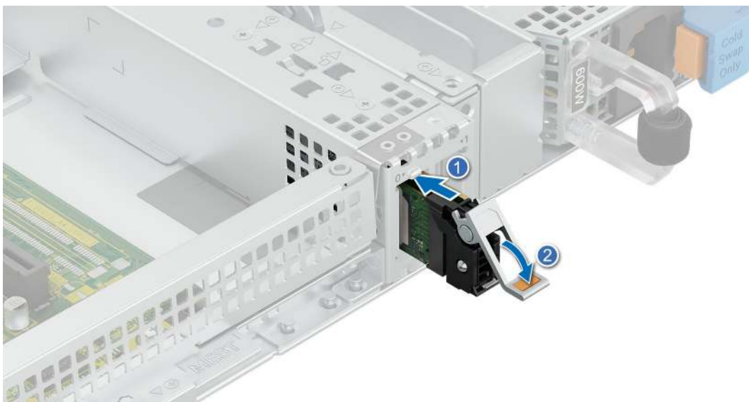
Figure 80. Installing the BOSS-N1 M.2 module
