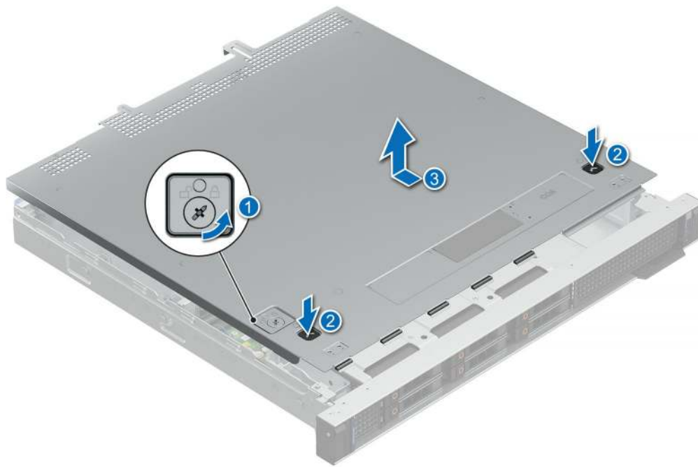
Figure 25. Removing the system cover
