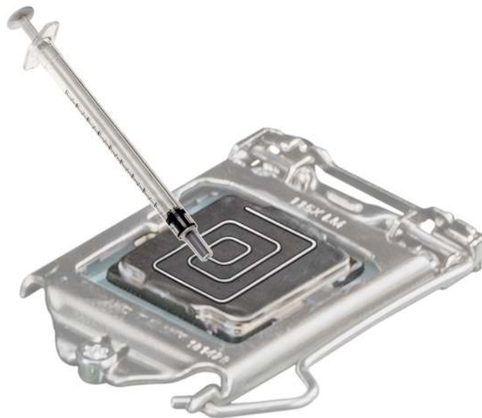
Figure 55. Applying thermal grease on top of the processor
