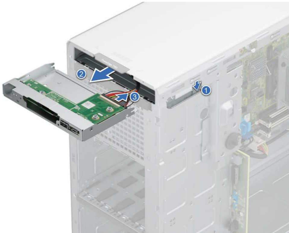
Figure 93. Removing the control panel cage
