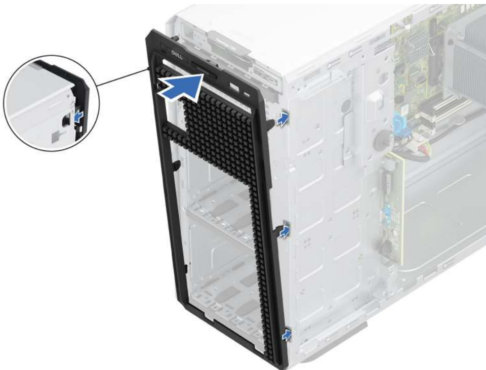
Figure 97. Installing the front faceplate
