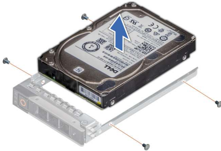
Figure 28. Removing the drive from the drive carrier
