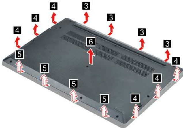
Figure 77. Pry up the latches and remove the lower case
