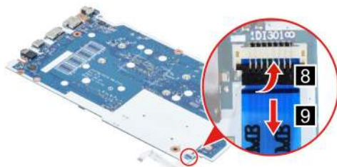
Figure 130. Disconnect the touchpad board cable from the system board
