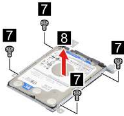
Figure 45. Remove four screws and then separate the HDD from the HDD bracket
