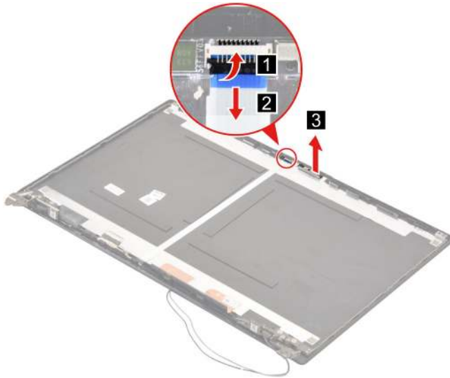
Figure 139. Disconnect the EDP cable from the camera board and then remove the camera
