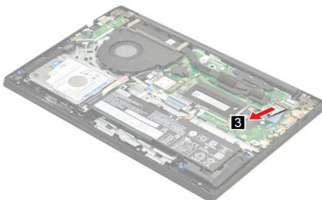
Figure 115. Remove the SSD by pulling it away from the slot
