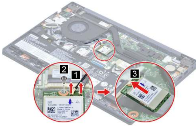
Figure 17. Remove the Wi-Fi card
