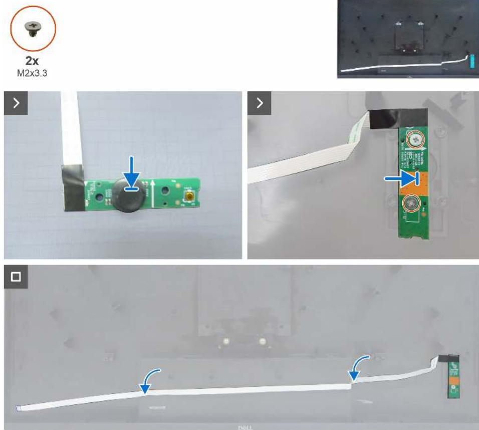
Figure 19. Installing the keypad board
