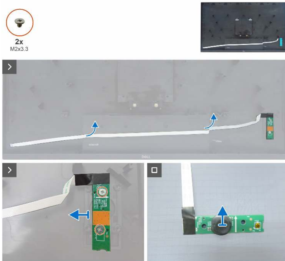
Figure 18. Removing the keypad board
