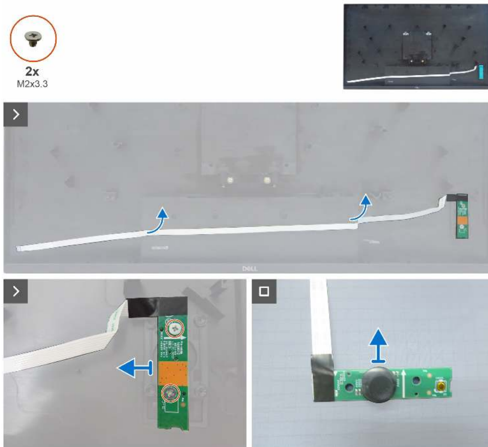
Figure 17. Removing the keypad board
