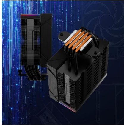
Single Tower Design with 4 Heat Pipes
