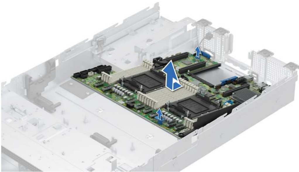
Figure 135. Removing the system board
