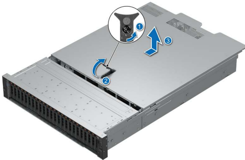
Figure 33. Removing the system cover
