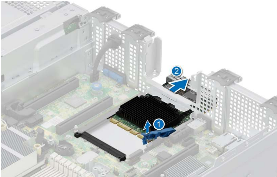
Figure 123. Removing the OCP card
