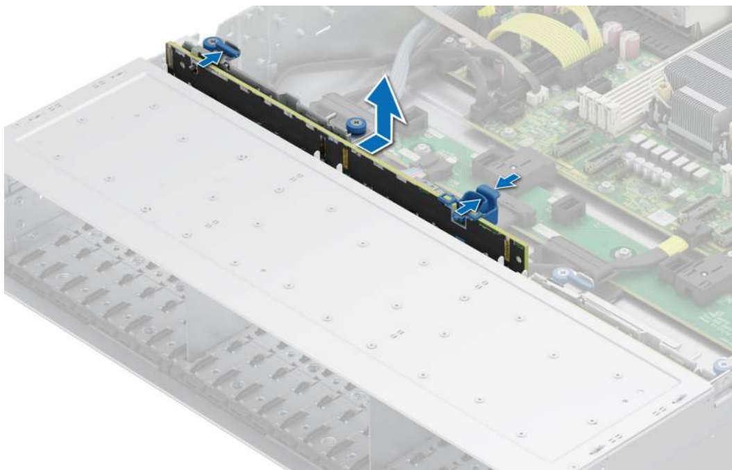
Figure 61. Removing the drive backplane
