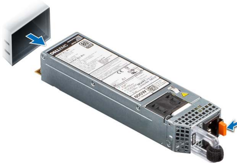
Figure 131. Removing a power supply unit
