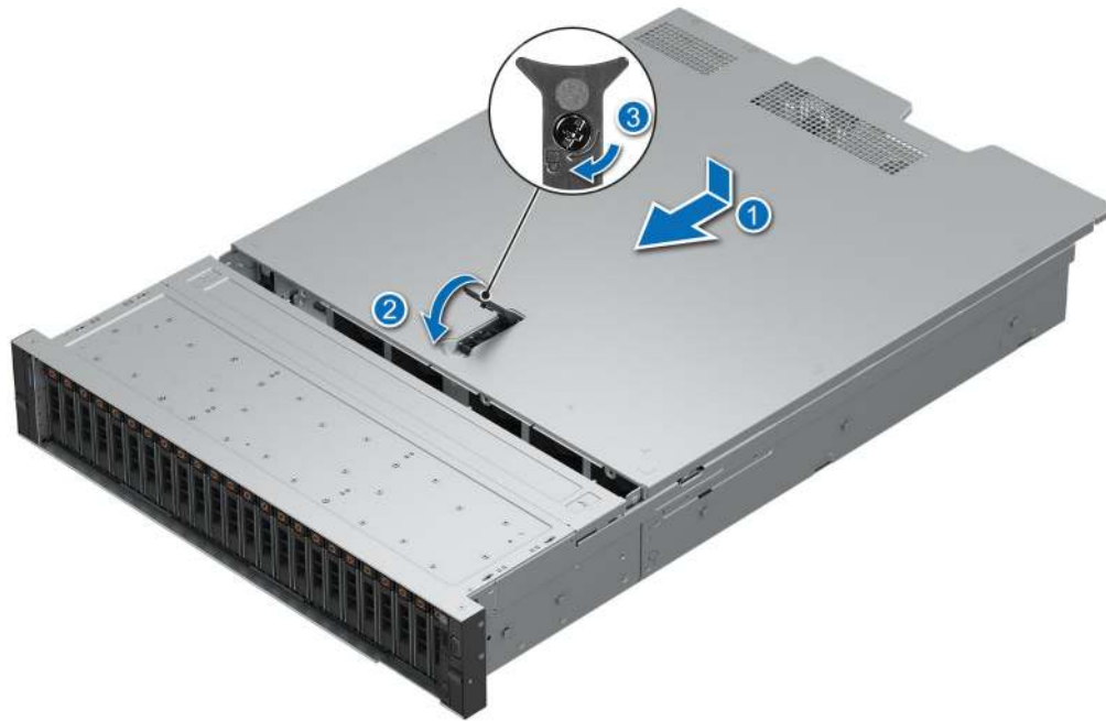
Figure 34. Installing the system cover
