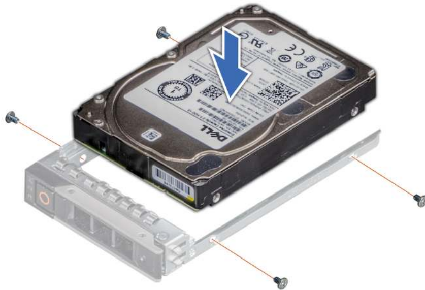
Figure 56. Installing a drive into the drive carrier
