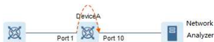
Figure 4-1 Operating Principle of Port Mirroring
