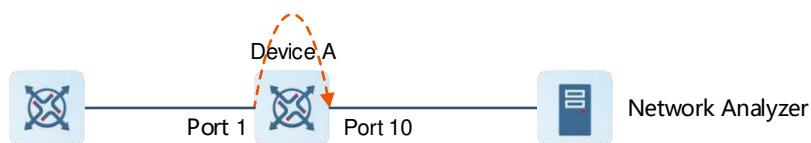
Figure 12-1 Port Mirroring Principles Figure
