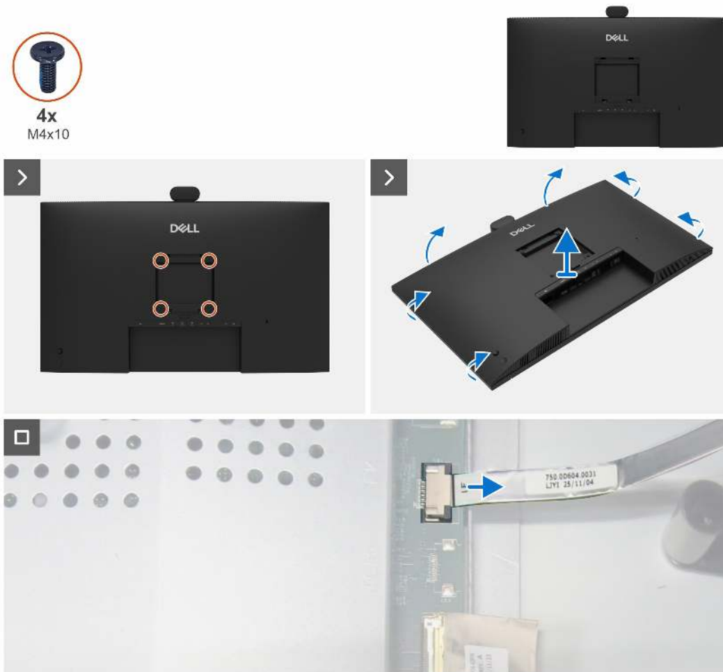
Figure 18. Removing the back cover
