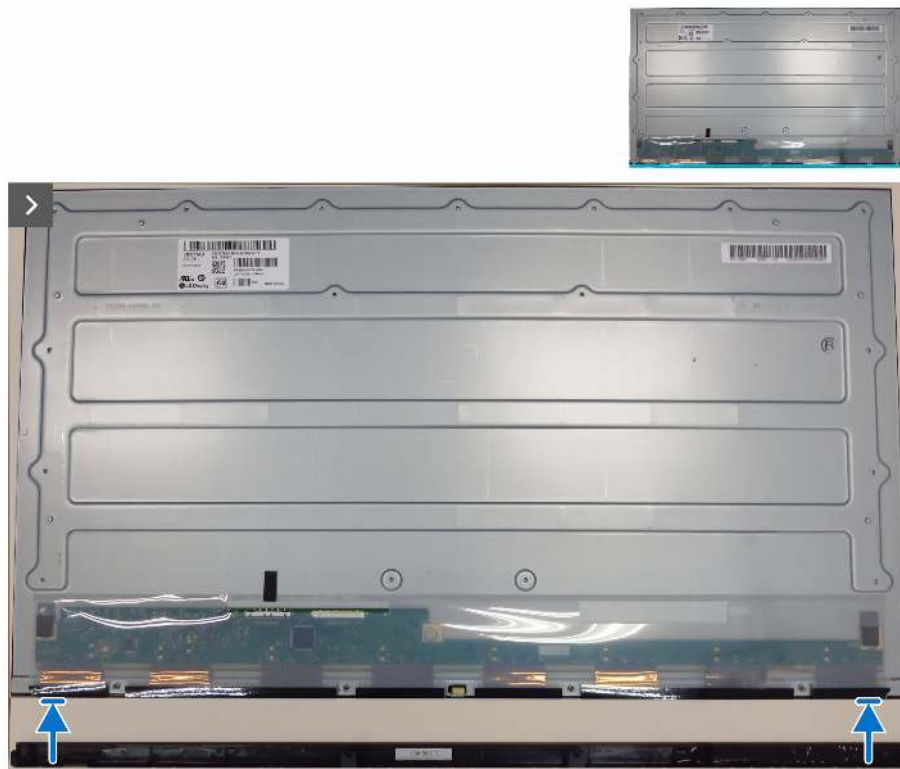
Figure 33. Installing the front trim
