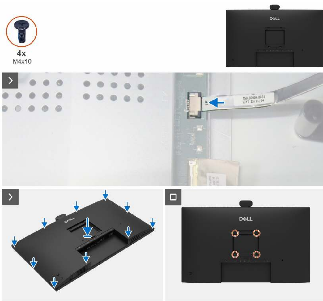
Figure 19. Installing the back cover
