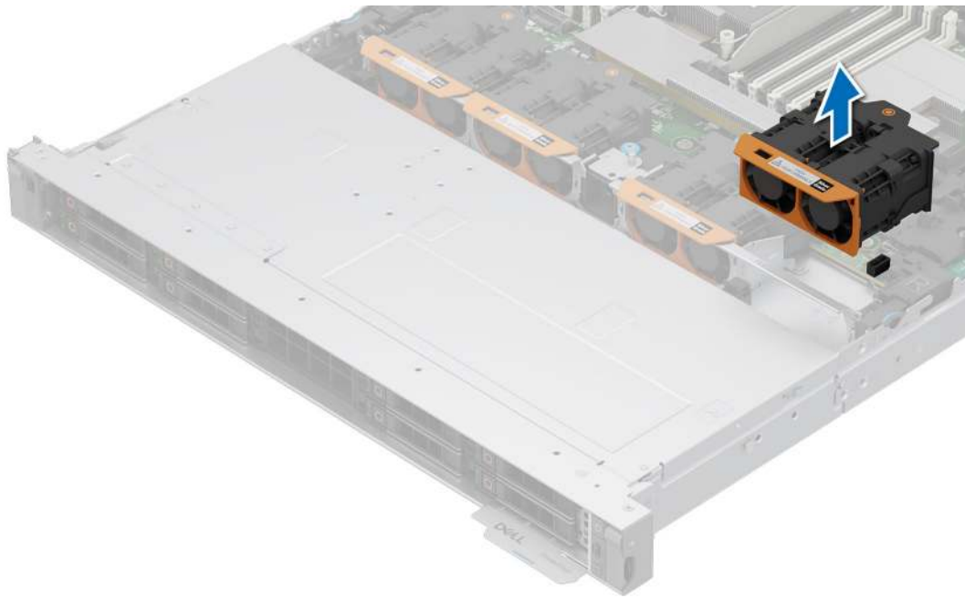
Figure 42. Removing a cooling fan
