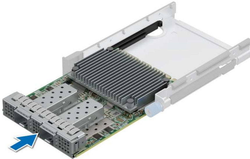
Figure 203. Installing the OCP NIC card into the OCP NIC card tray
