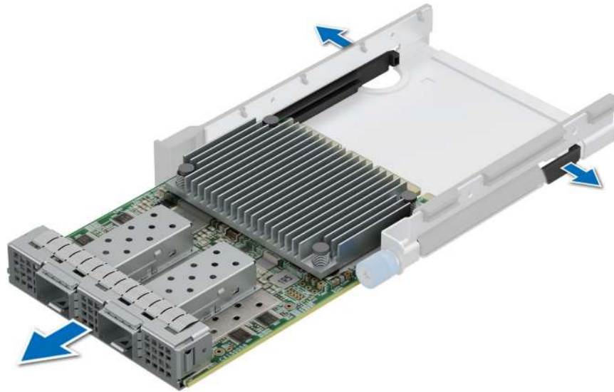
Figure 201. Removing the OCP NIC card from the tray
