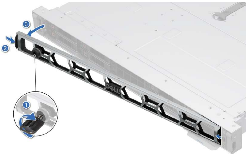
Figure 36. Removing the front bezel
