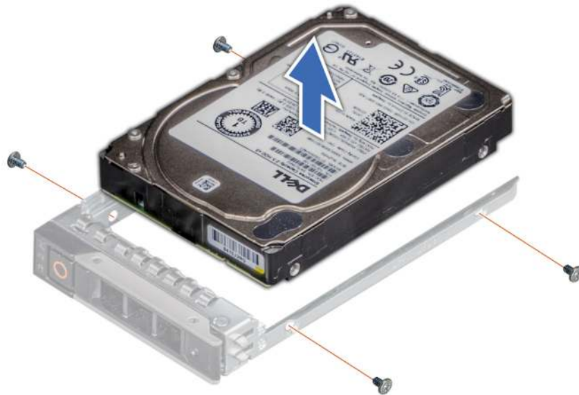
Figure 61. Removing the 3.5-inch drive from the drive carrier
