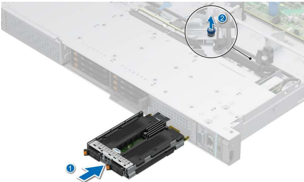
Figure 195. Installing the BOSS-N1 DC-MHS module tray into system
