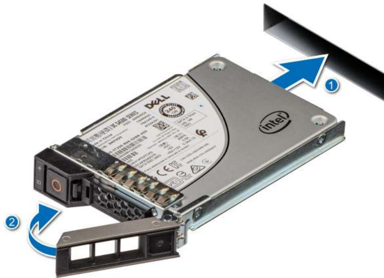
Figure 57. Installing a 2.5-inch drive carrier
