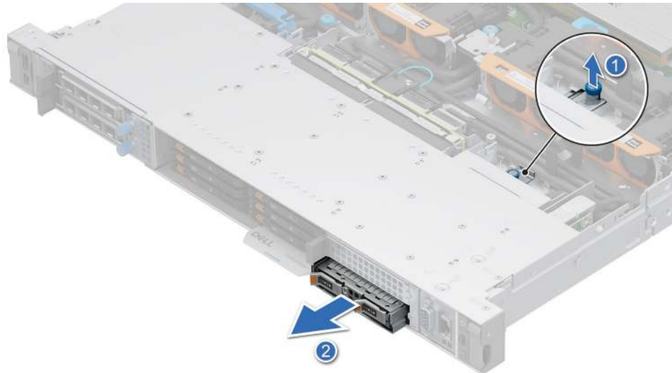
Figure 189. Removing an BOSS-N1 DC-MHS module tray from the system
