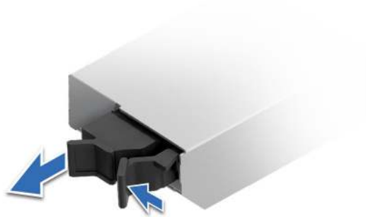
Figure 186. Removing the BOSS-N1 DC-MHS card carrier blank
