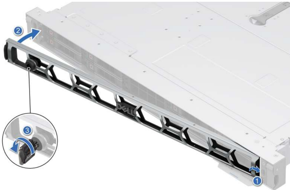
Figure 37. Installing the front bezel
