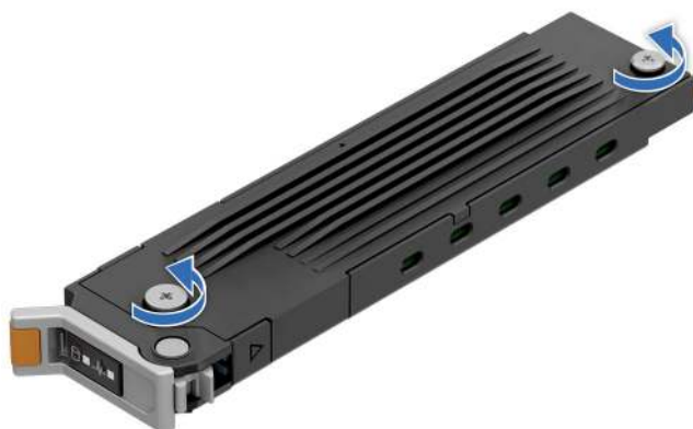
Figure 167. Loosen the top cover captive screws
