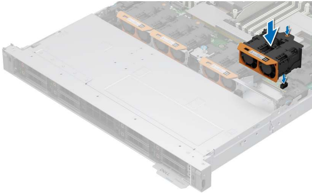
Figure 43. Installing a cooling fan
