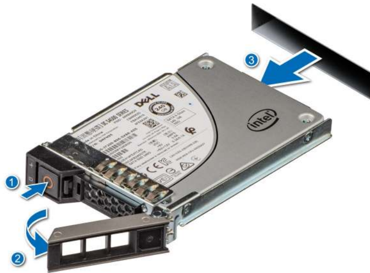
Figure 54. Removing a 2.5-inch drive carrier
