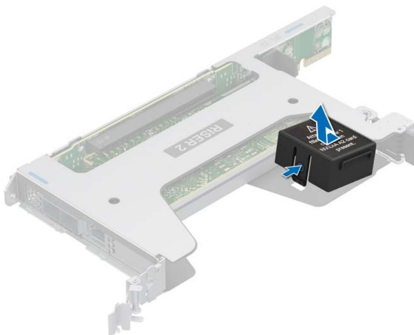
Figure 135. Removing GPU blank from the rear expansion card riser 2q
