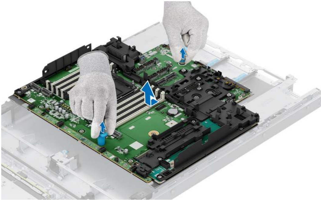
Figure 231. Removing the HPM board
