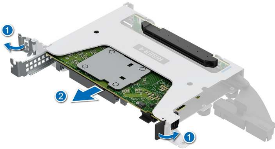
Figure 136. Removing expansion card from the rear expansion card riser 4b
