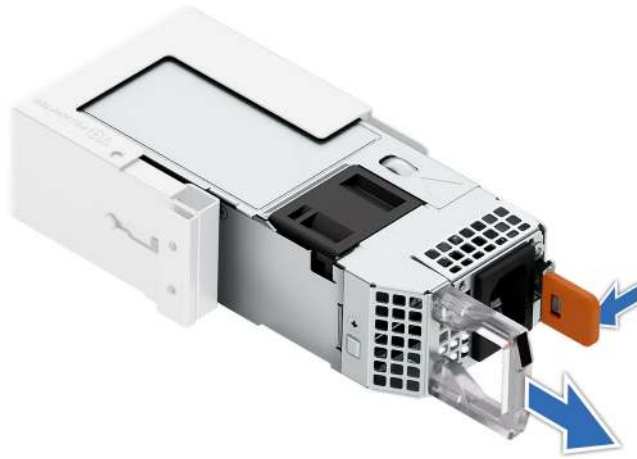
Figure 225. Removing a power supply unit
