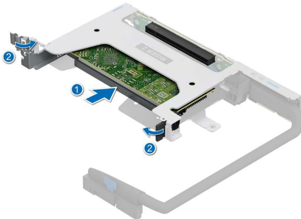
Figure 147. Installing an expansion card into the riser 2q
