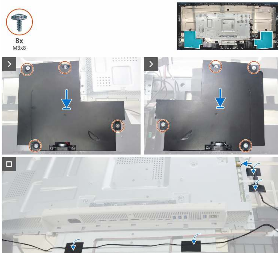
Figure 28. Installing the speakers
