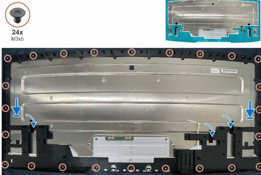
Figure 34. Installing the middle frame
