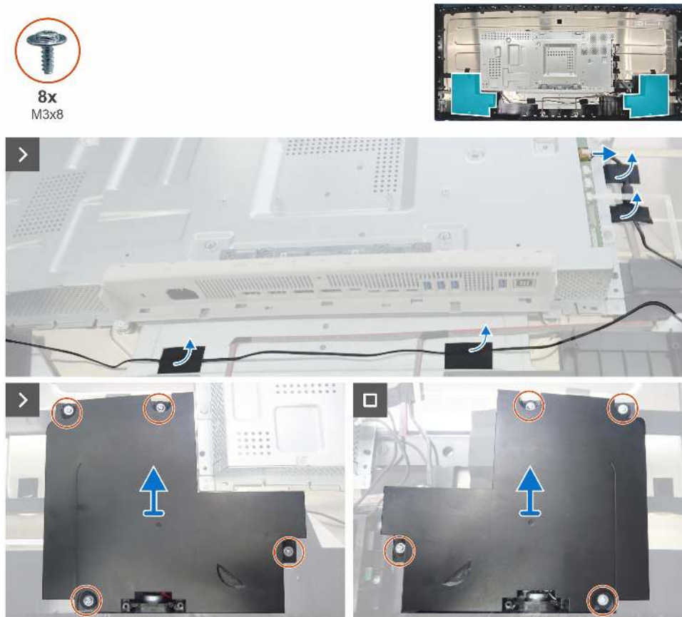
Figure 27. Removing the speakers
