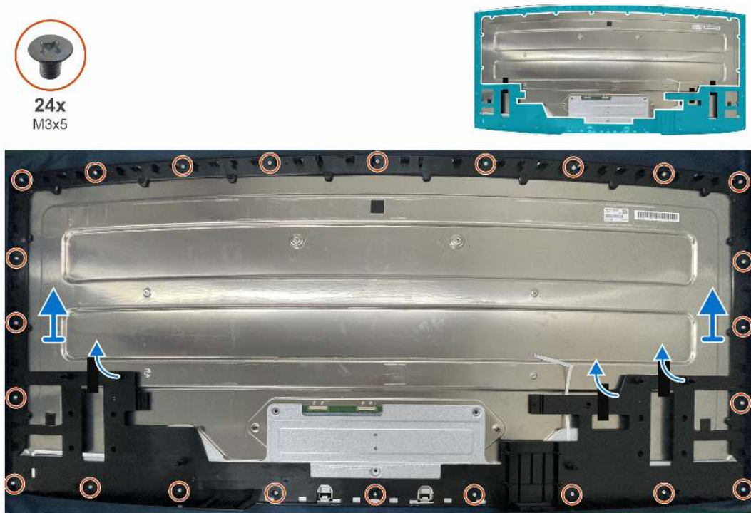
Figure 33. Removing the middle frame
