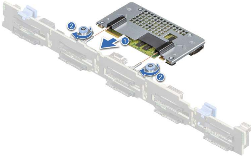
Figure 117. Installing the rear mounting front PERC module
