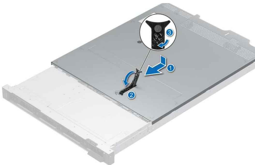
Figure 24. Installing the system cover
