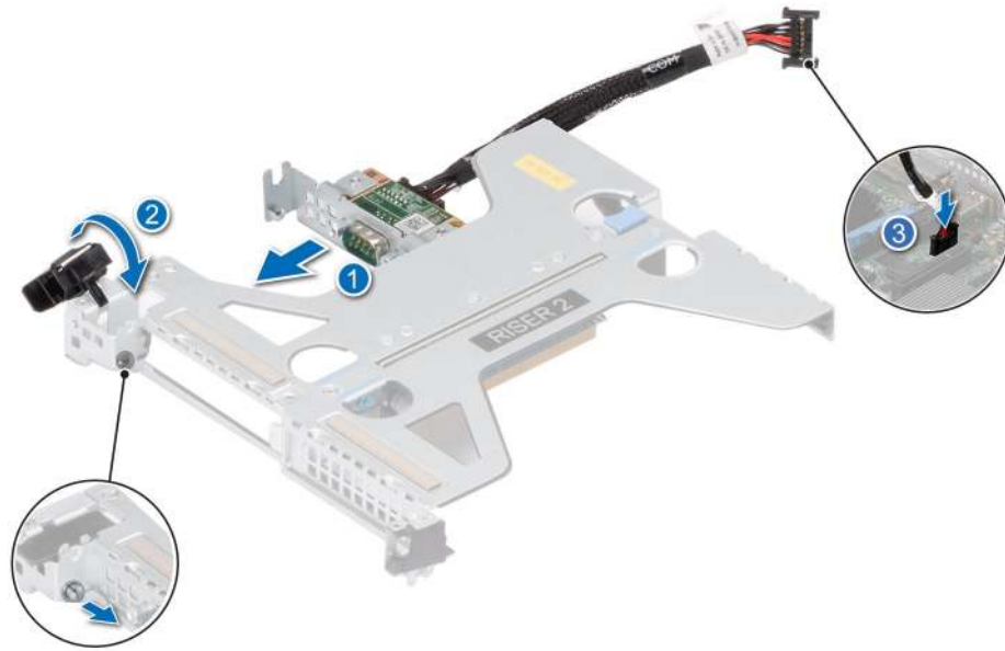
Figure 105. Installing the Serial COM port
