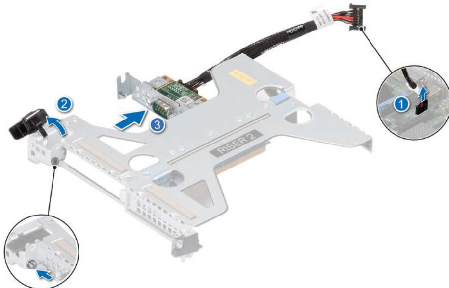
Figure 102. Removing the Serial COM port
