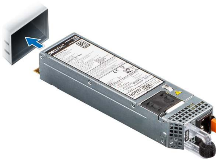
Figure 127. Installing a power supply unit
