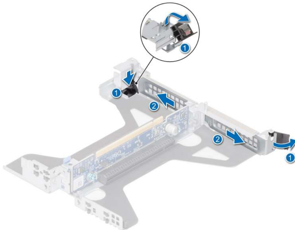
Figure 97. Removing filler bracket from Riser 2a
