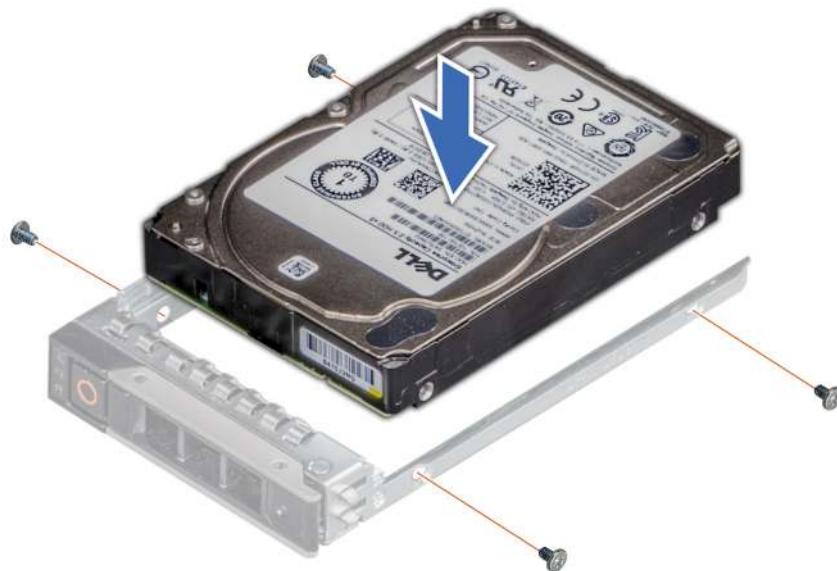
Figure 38. Installing a drive into the drive carrier
