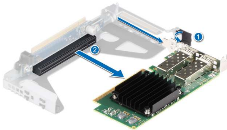
Figure 92. Removing an expansion card from the Riser 1a
