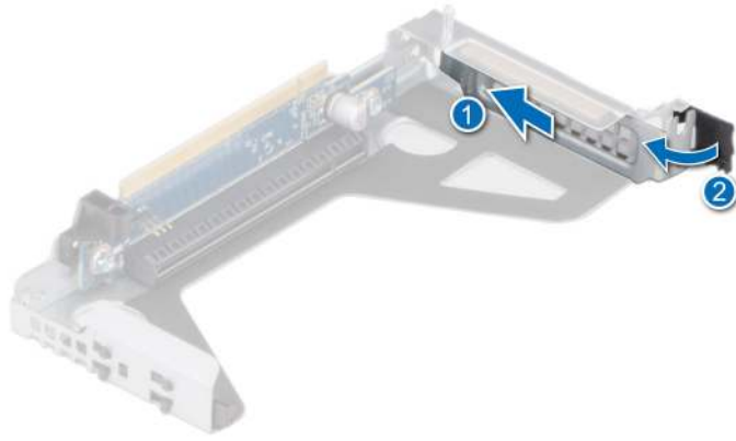
Figure 94. Installing filler bracket in the Riser 1a/1b
