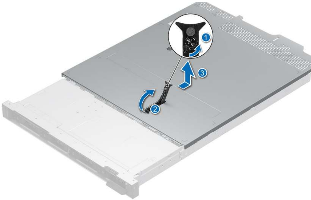
Figure 23. Removing the system cover
