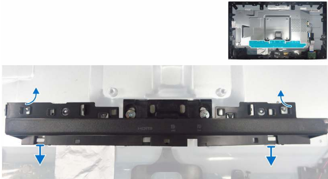
Figure 18. Removing the I/O cover
