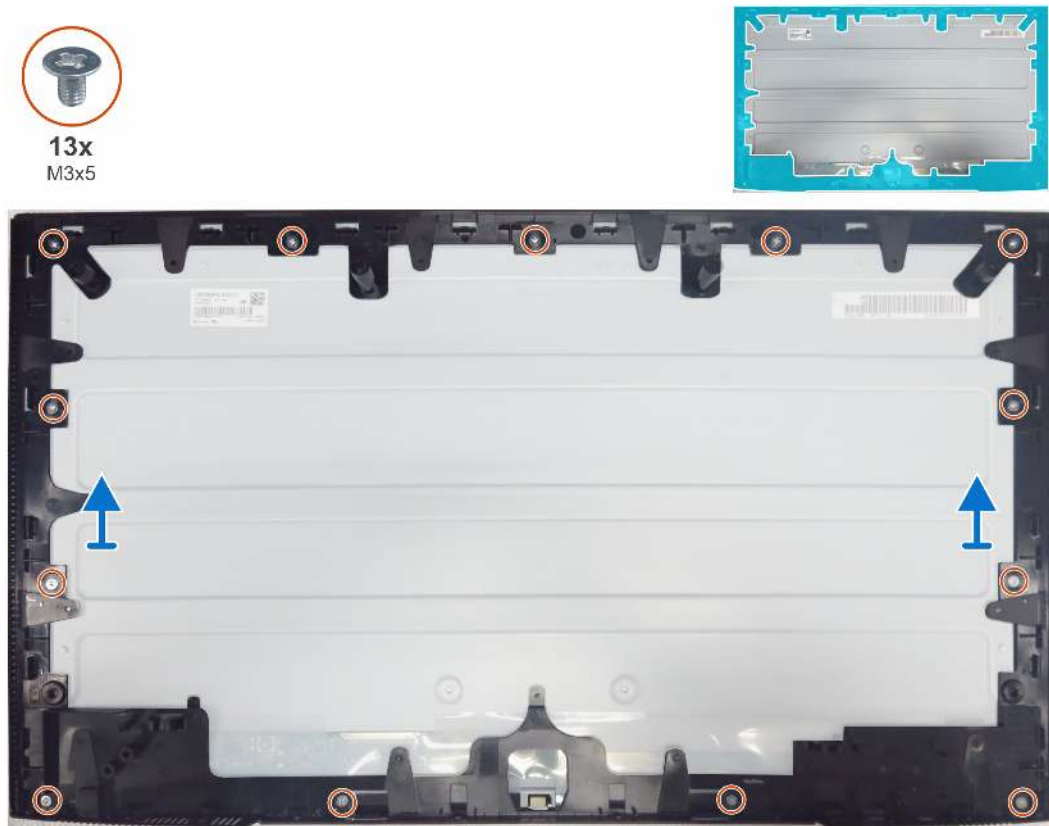
Figure 24. Removing the middle frame
