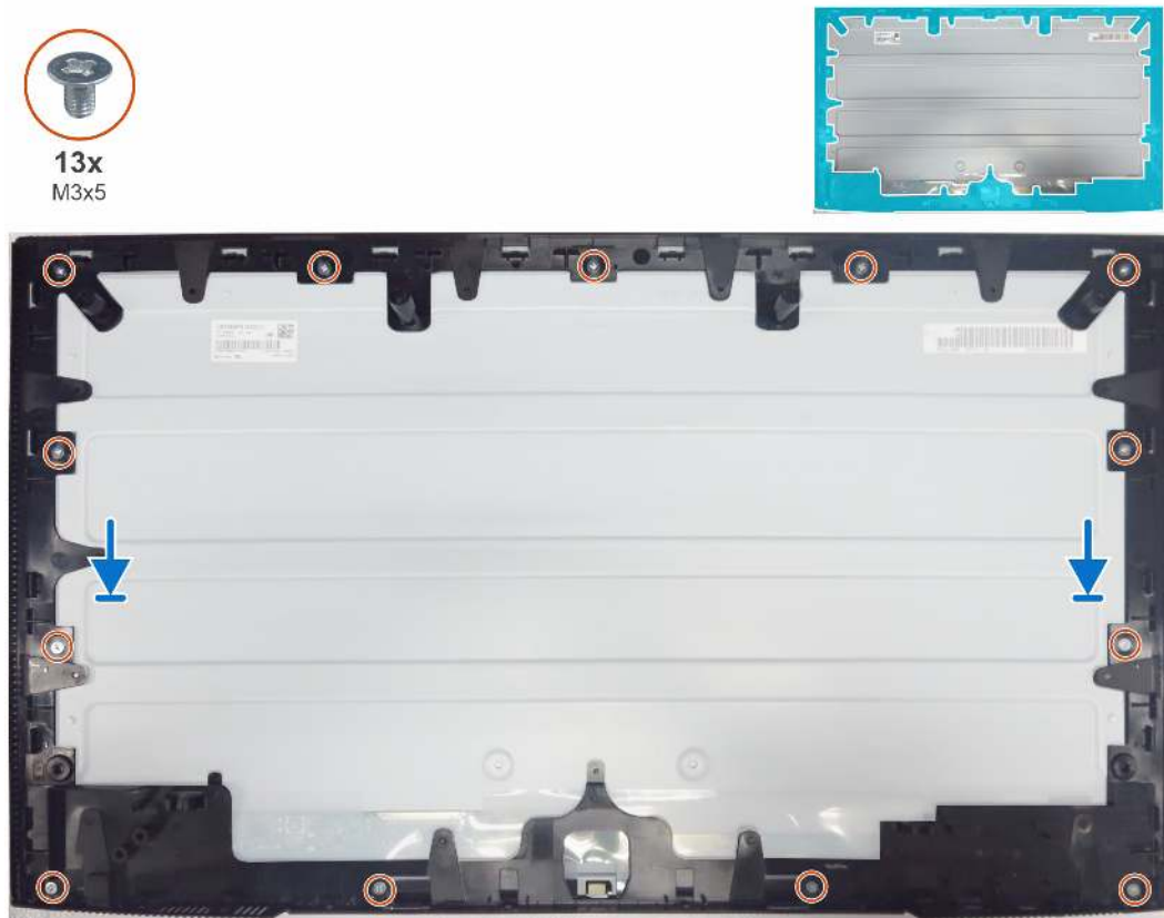
Figure 25. Installing the middle frame
