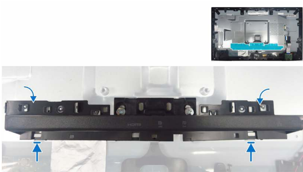
Figure 19. Installing the I/O cover
