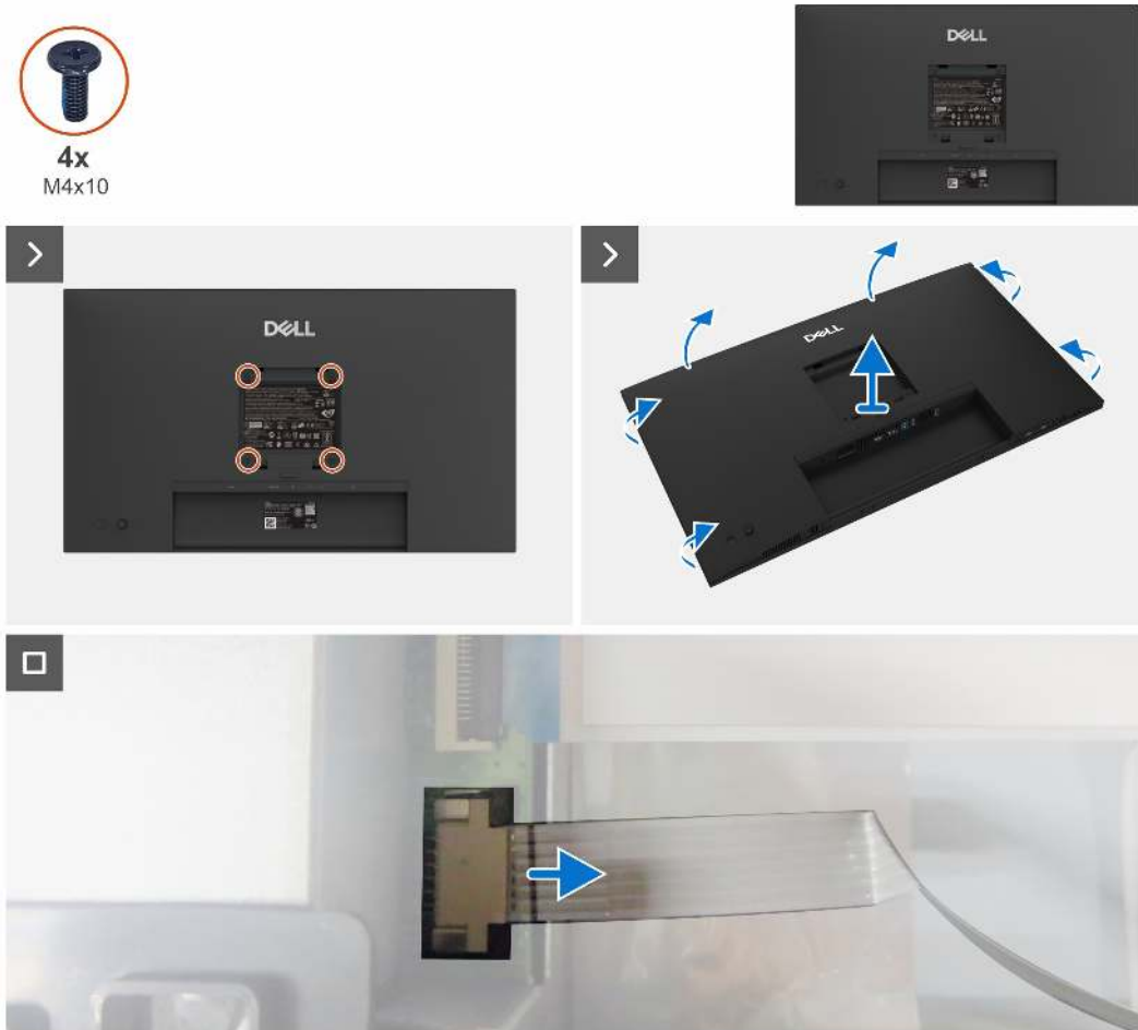
Figure 10. Removing the back cover
