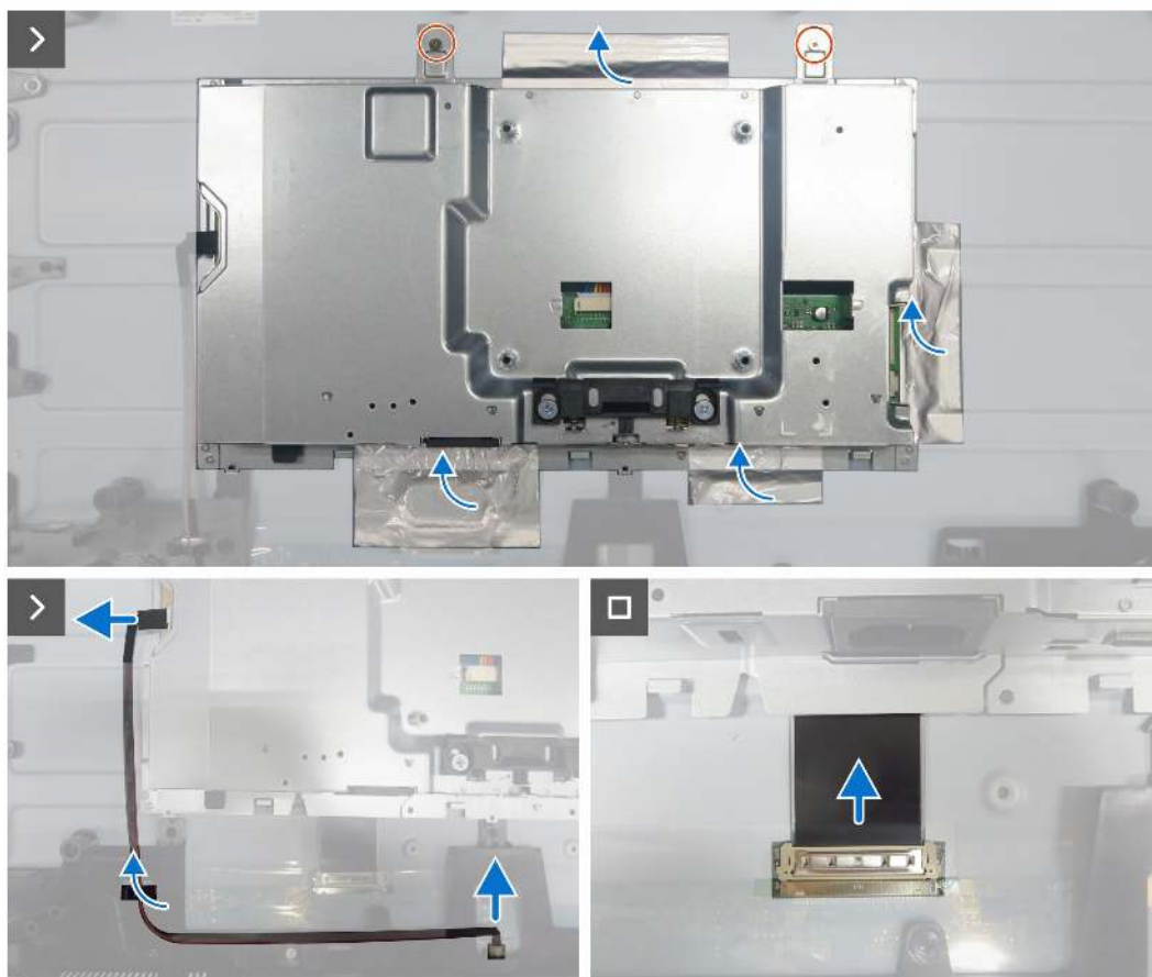
Figure 18. Removing the main chassis
