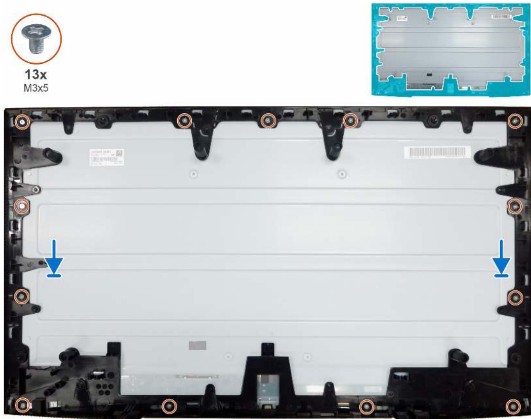
Figure 21. Installing the middle frame
