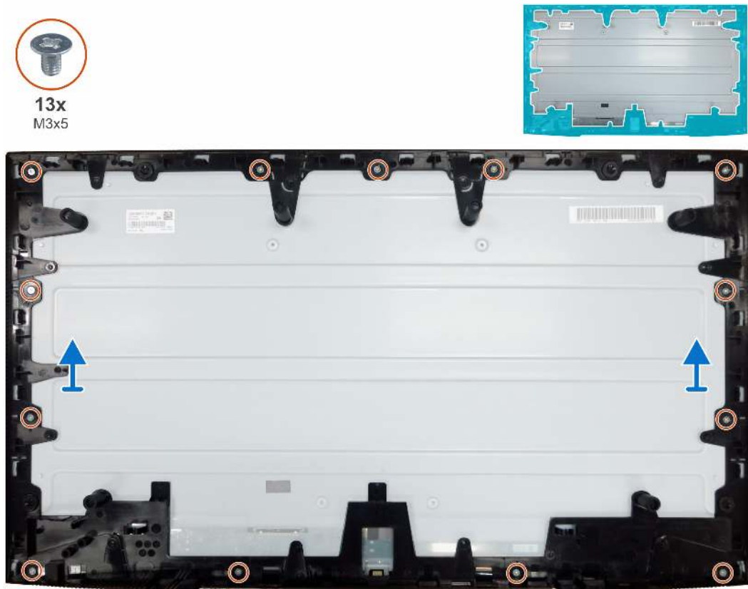
Figure 20. Removing the middle frame
