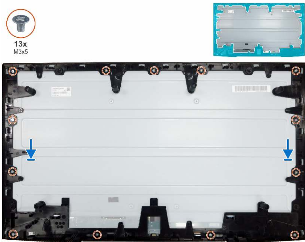
Figure 21. Installing the middle frame
