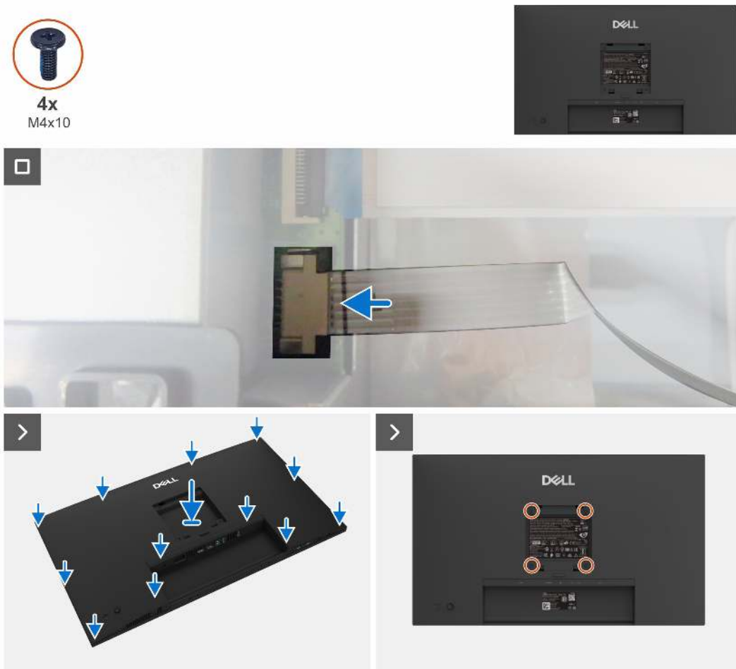
Figure 11. Installing the back cover
