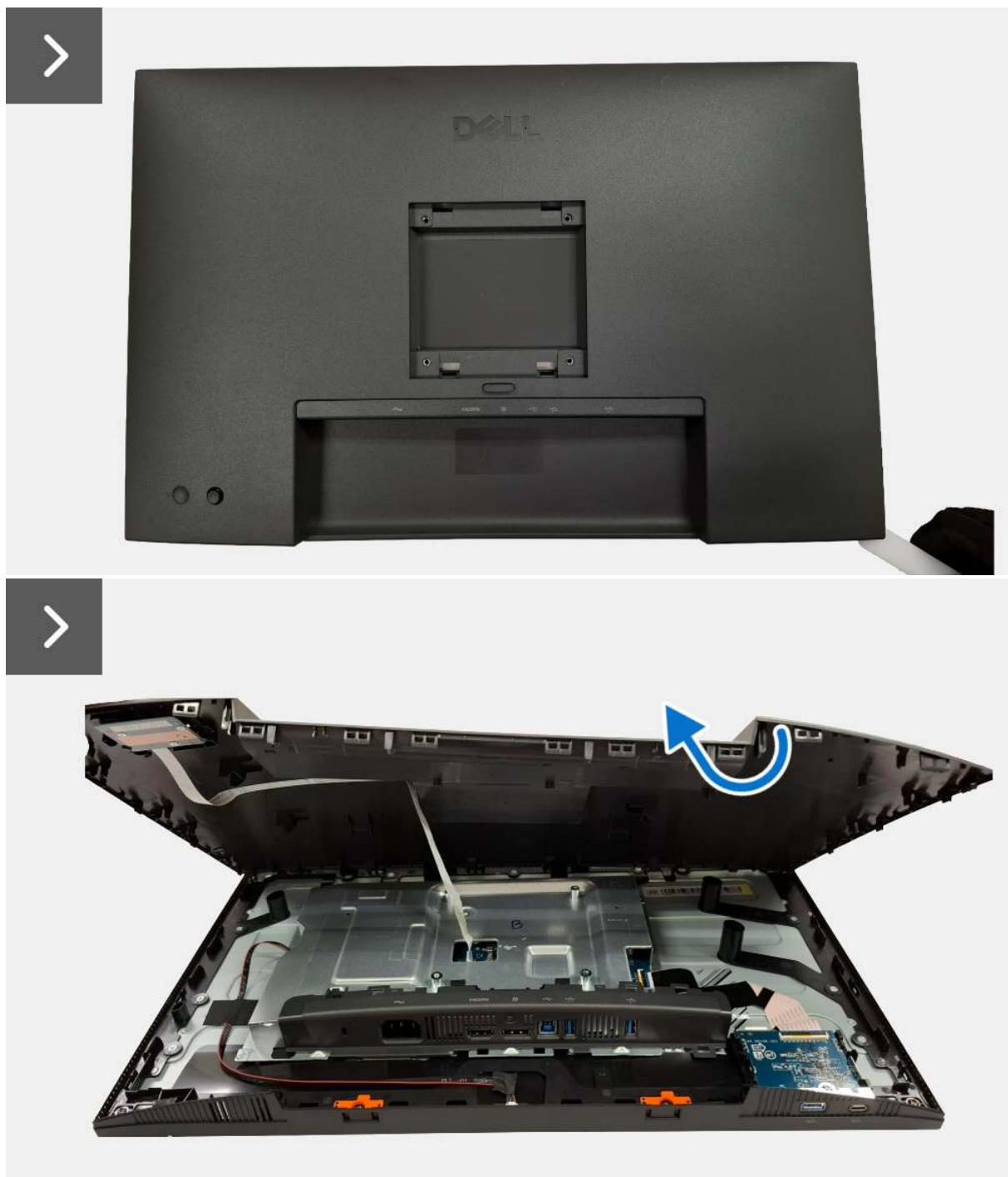
Figure 13. Removing the back cover
