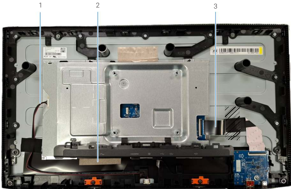
Figure 6. Wiring connectivity on display assembly
