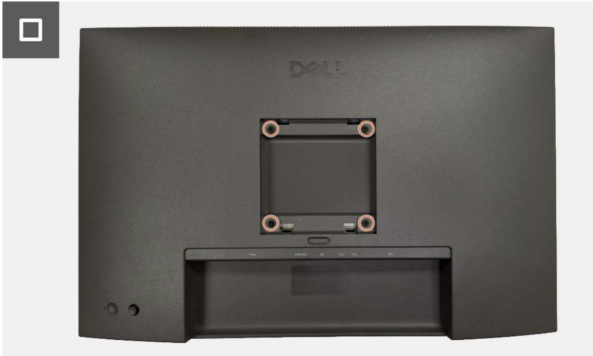
Figure 16. Installing the upper back cover
