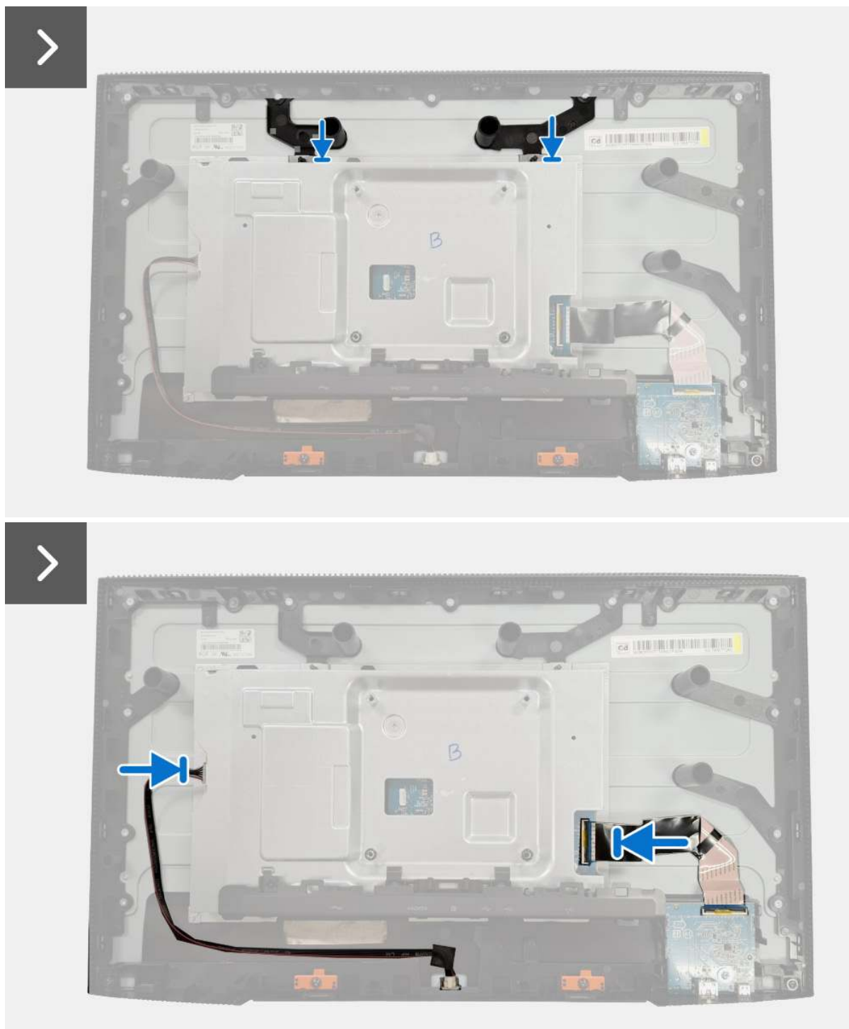
Figure 23. Installing the metal shield
