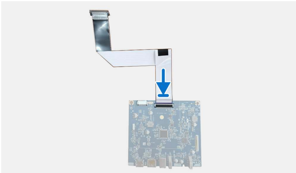
Figure 32. Installing the interface board
