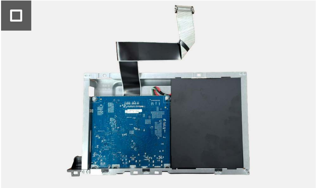
Figure 20. Removing the metal shield
