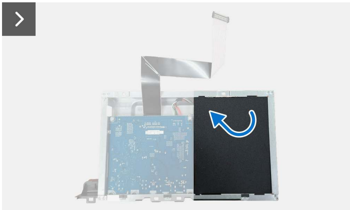
Figure 25. Removing the power board
